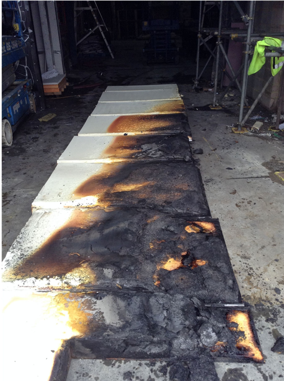
Figure 17. Photograph showing the condition of the insulation layer post-test (Insulation Layer removed from cladding wall).
