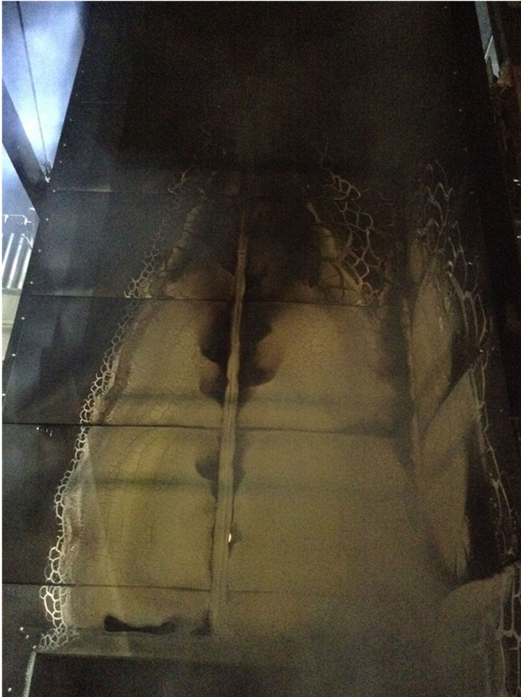
Figure 14. Photograph showing the condition of the cladding system post-test (Decorative Layer Full height).
