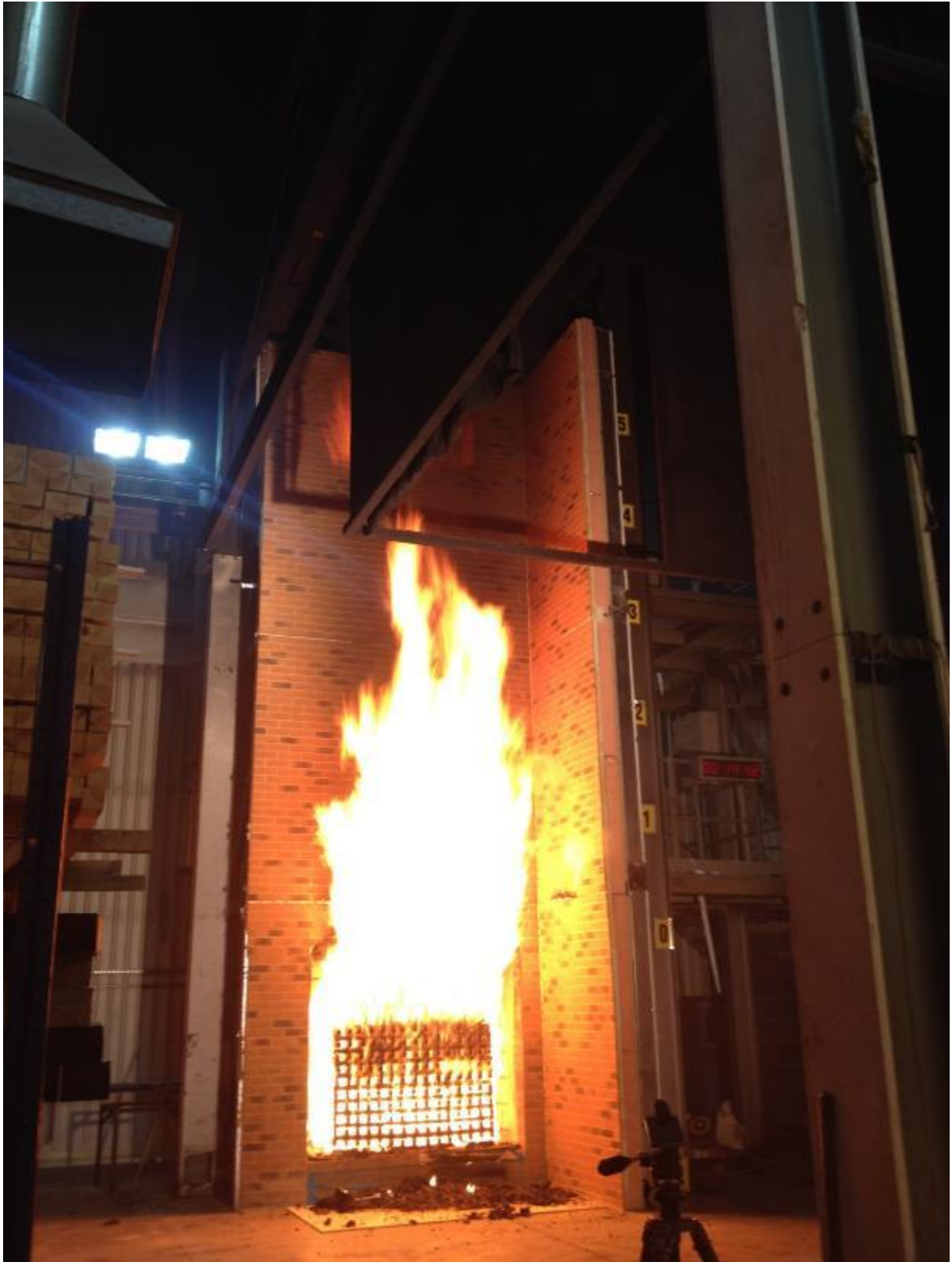
Figure 15. Cladding system during the test.
