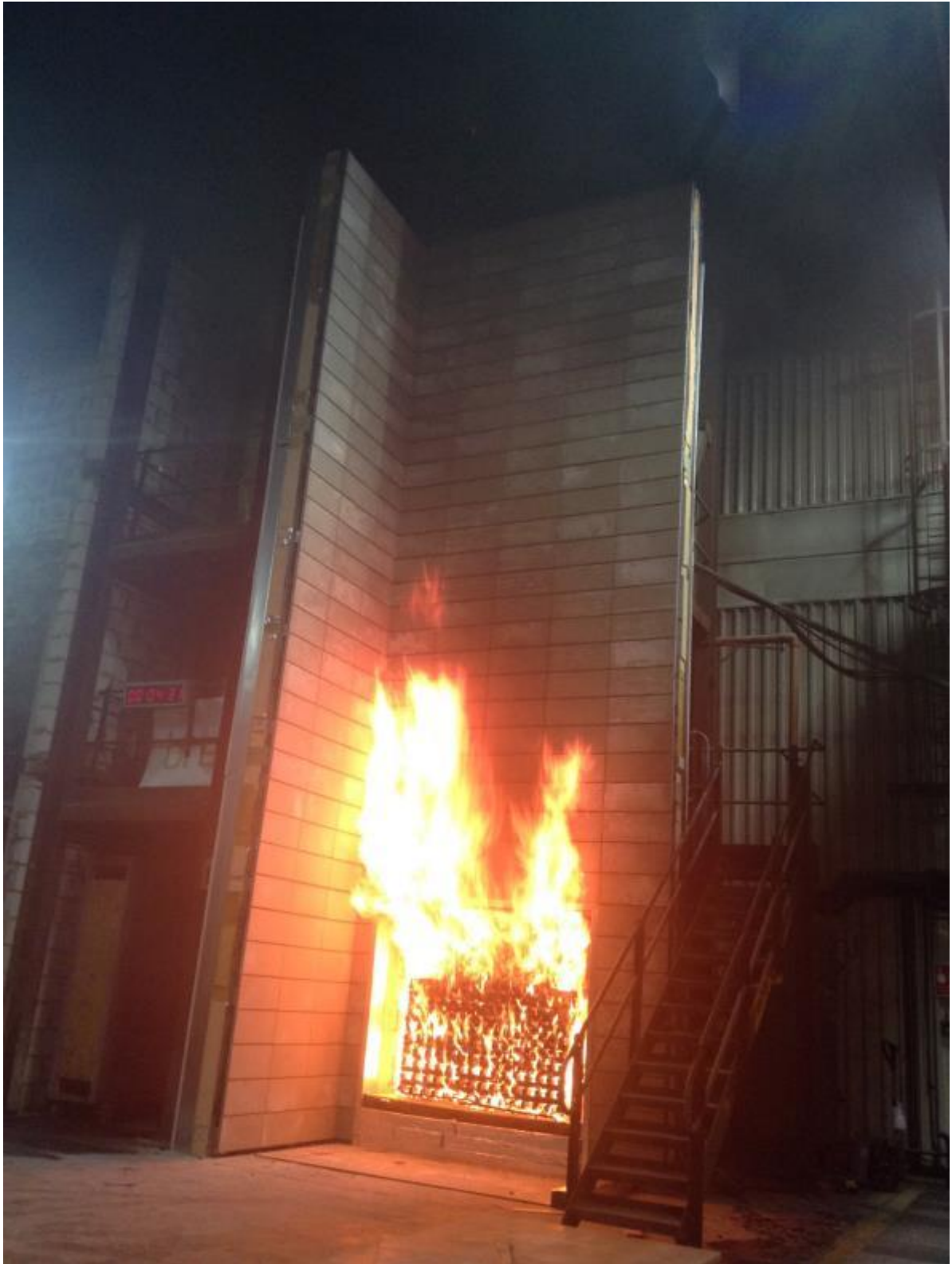
Figure 15. Cladding system during the test.
