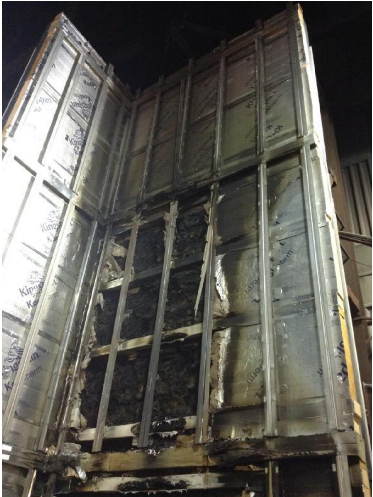
Figure 17. Photograph showing the condition of the insulation layer of the System post-test (Decorative layer removed)
