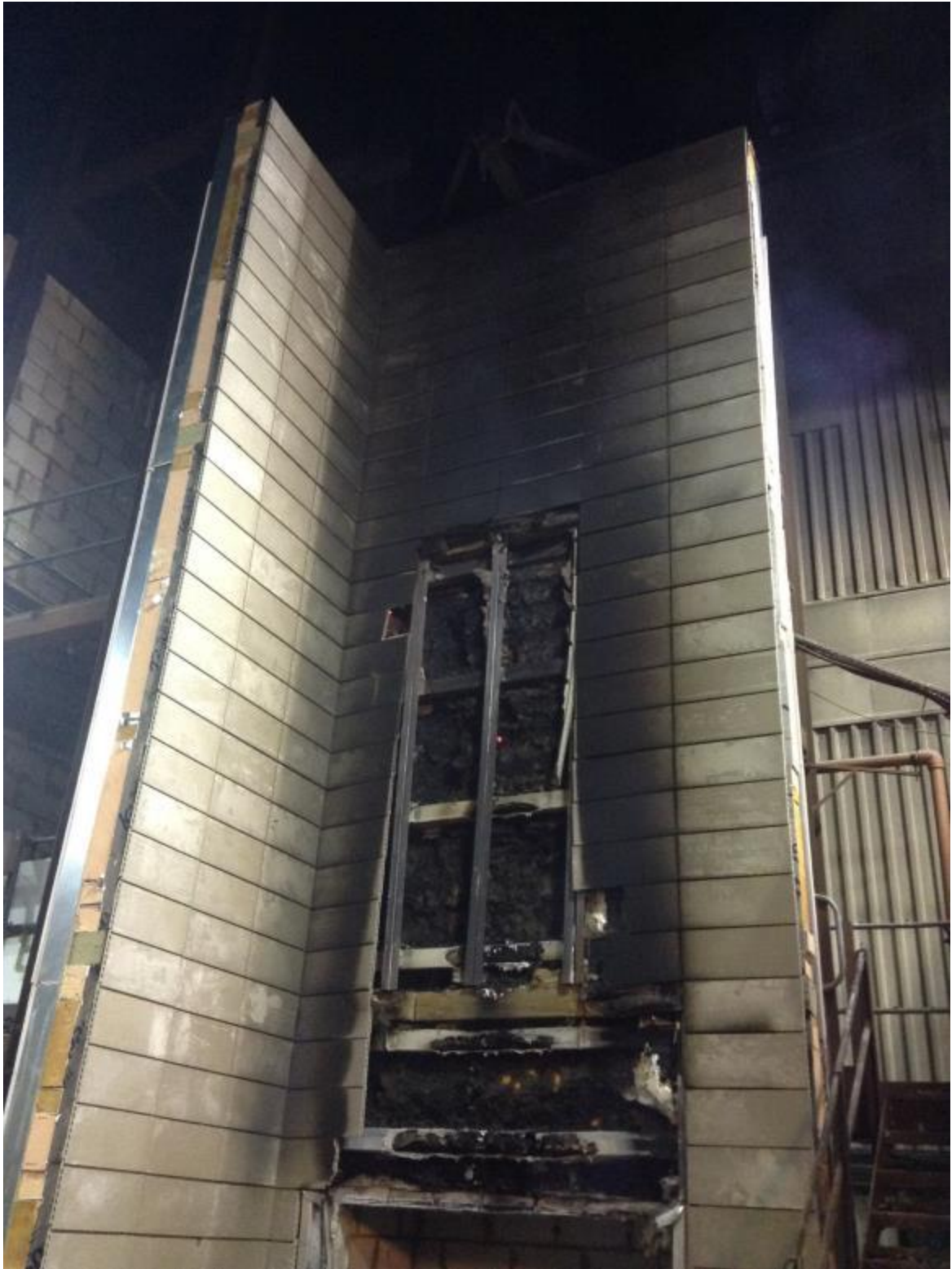
Figure 16. Photograph showing the condition of the cladding system post-test (Decorative Layer Full height).
