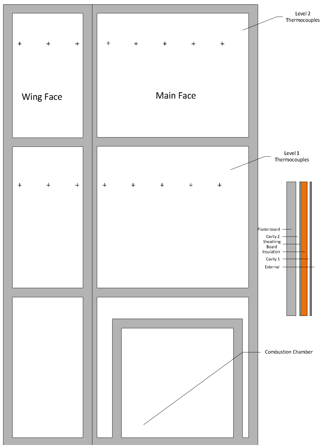
Figure 7. Locations of thermocouples used (schematic only)
