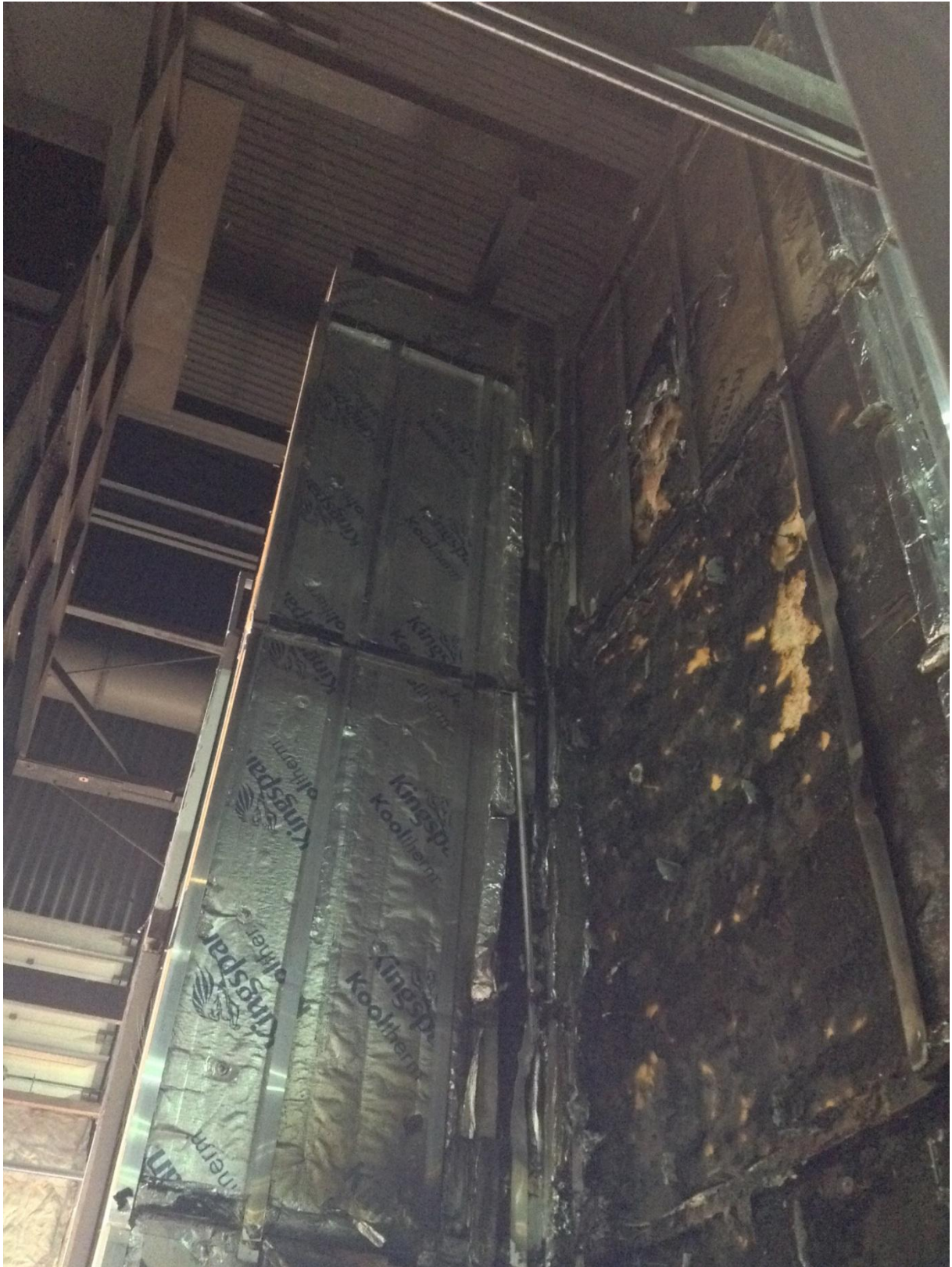
Figure 19. Tested system on completion of the test (2)
