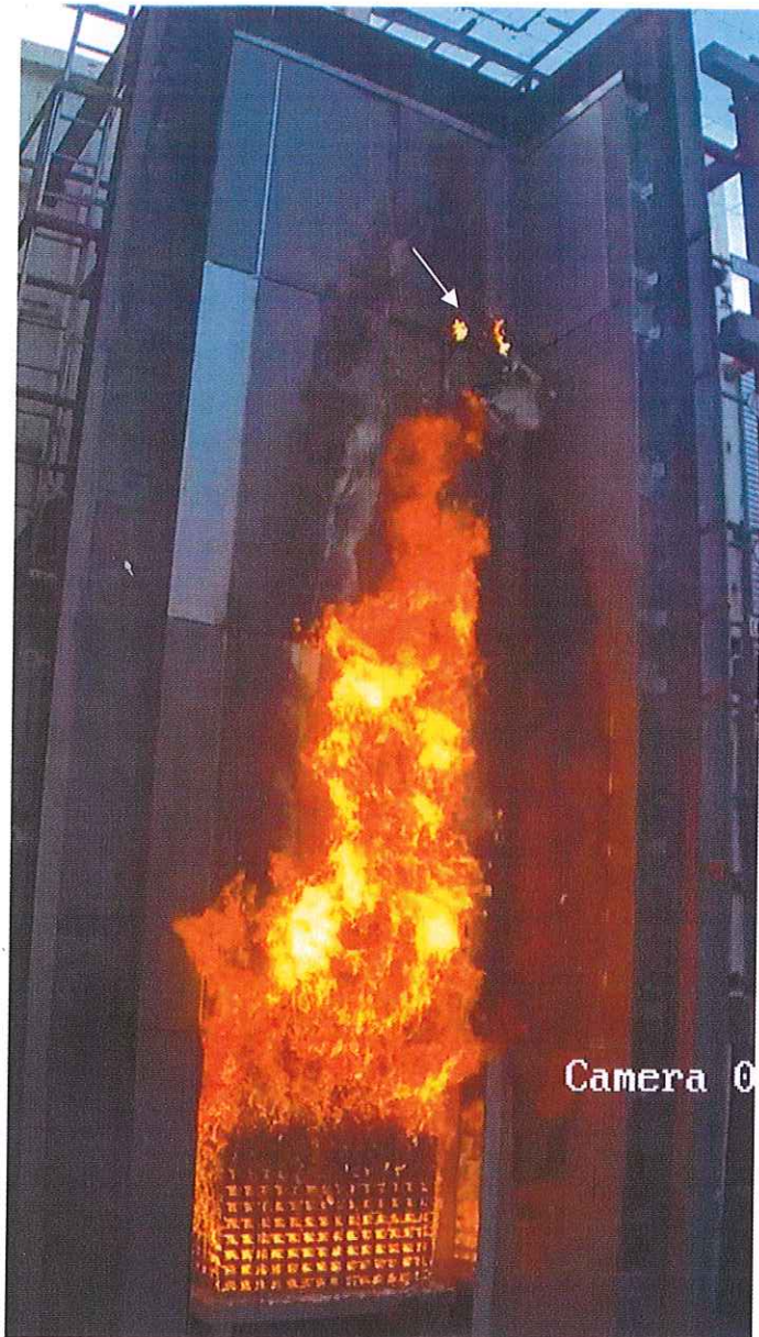
DLP C2753H/0006 Horizontal cavity barrier behind the panels M9 & M10 burning.
