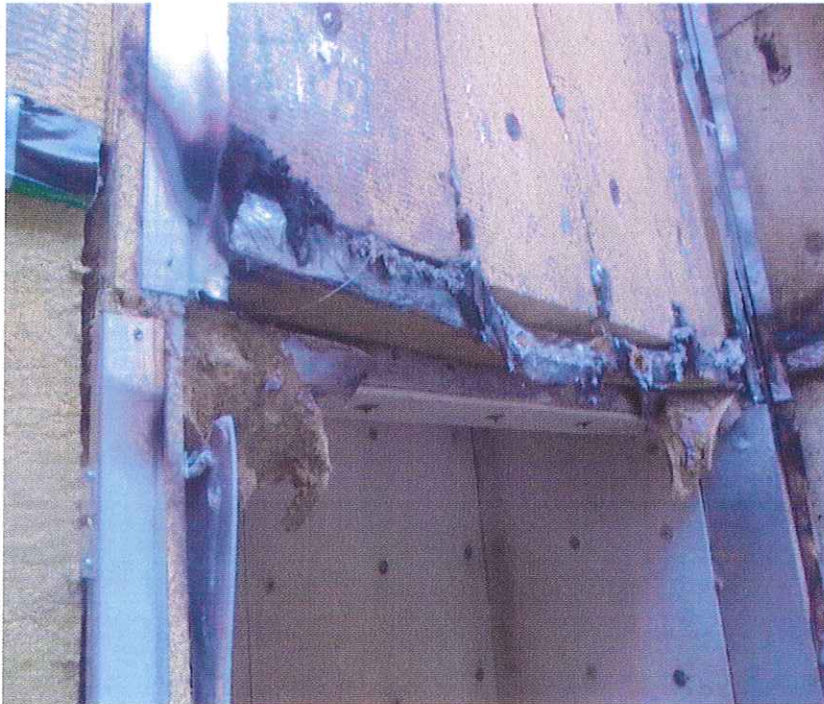
DLP C2753H/0012 Cavity barrier at the top of combustion chamber
