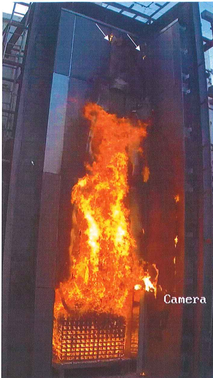
DLP C2753H/0007 Sporadic flame on panels M12, M13 & M14 vertical joints.
