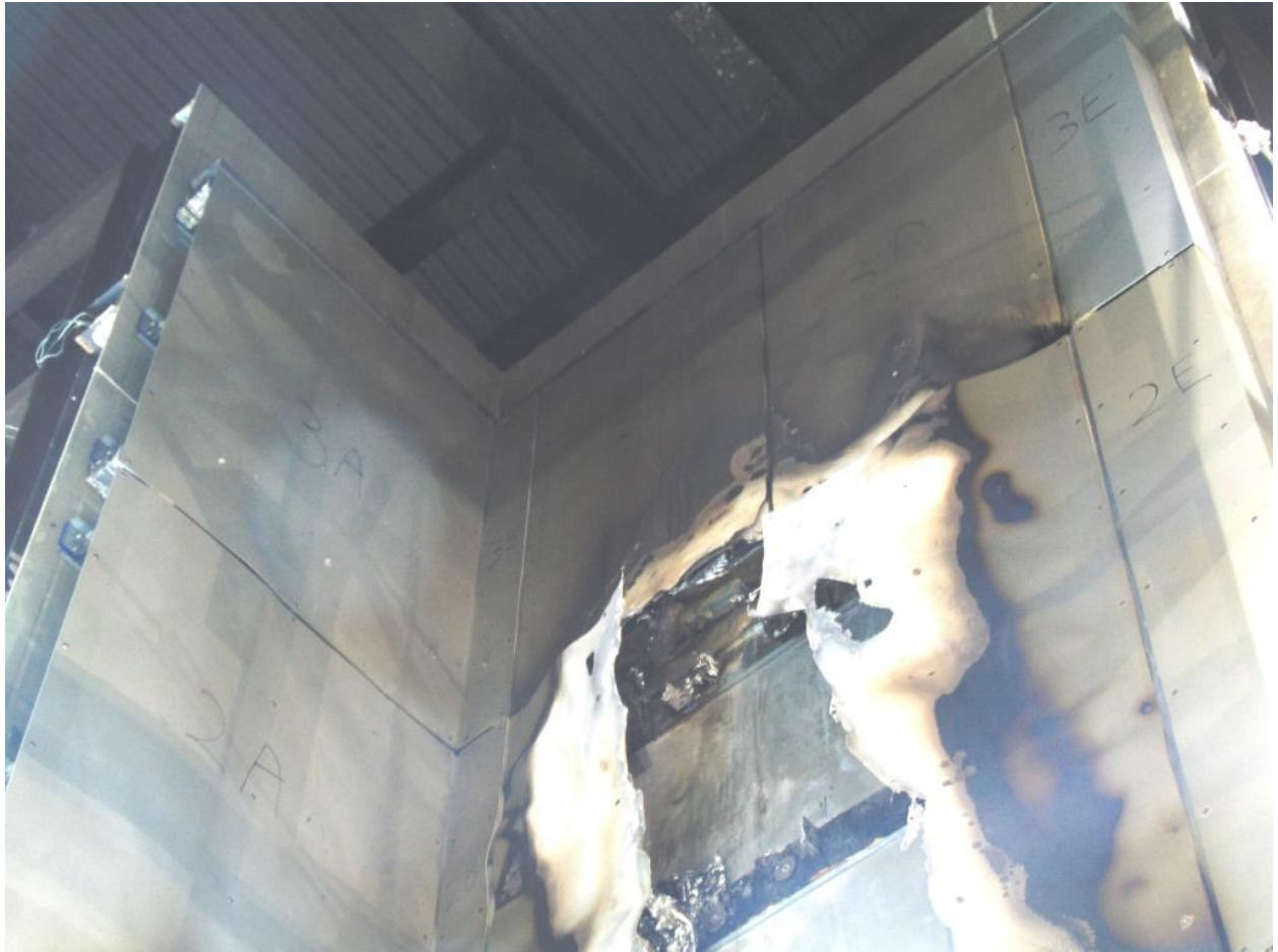
Figure 24. Damage to panels between a height of approximately 6000mm above the top of the combustion chamber and the top of the cladding system.
