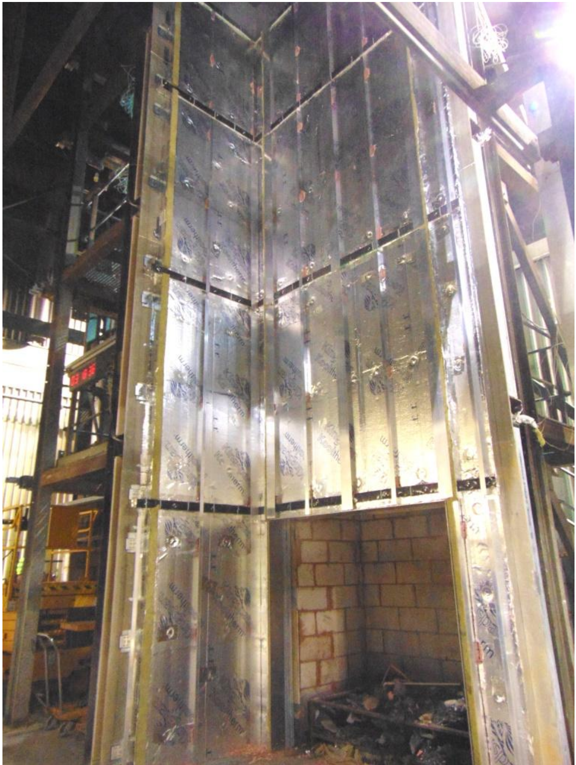
Figure 8. Vertical rails fitted to system.
