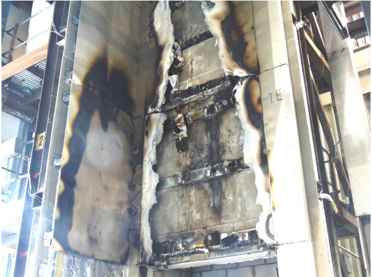
Figure 22. Damage to panels between top of combustion chamber and a height of approximately 5000mm above the top of the combustion chamber.
