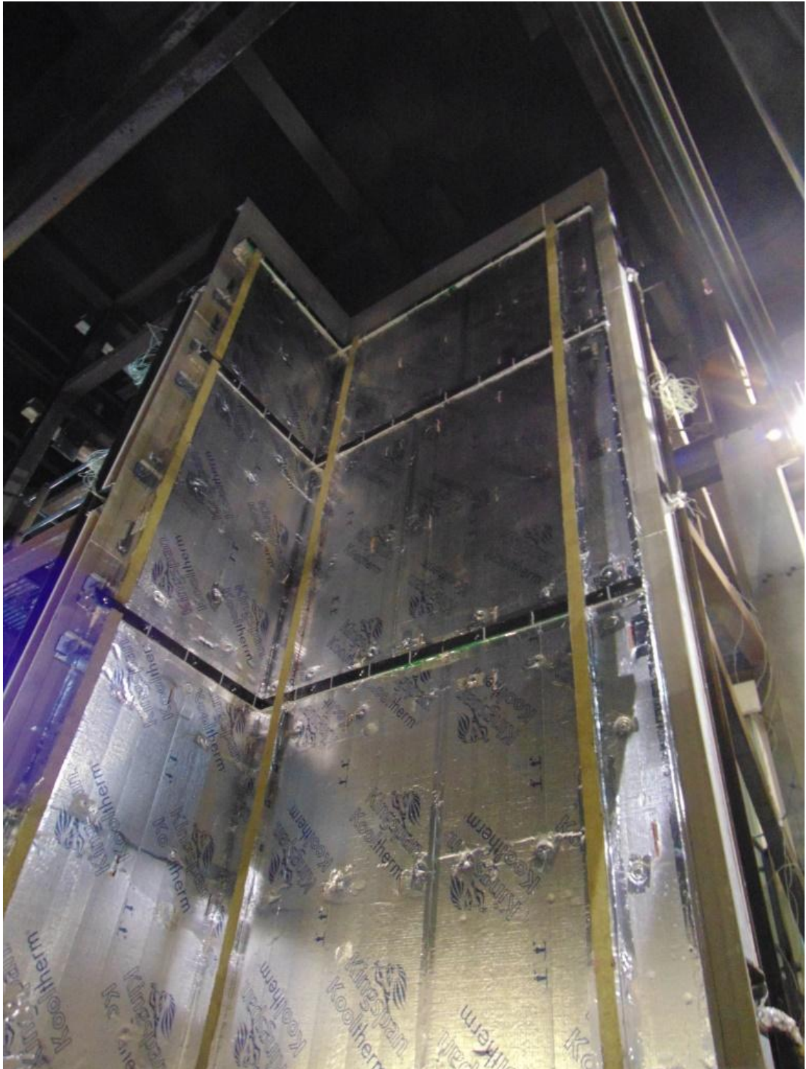
Figure 7. Insulation and cavity barriers fitted to system.
