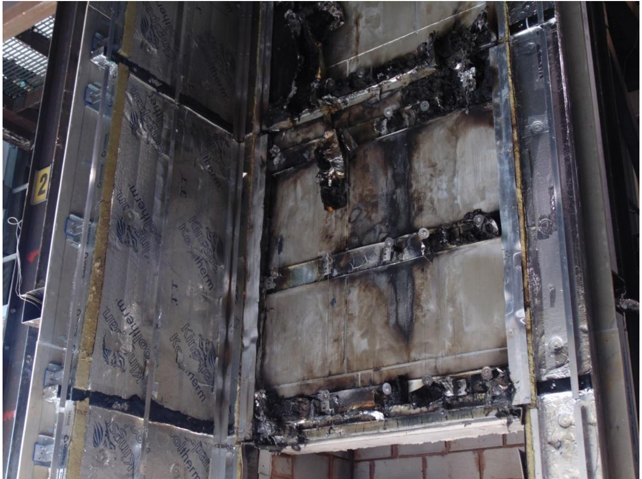
Figure 27. Damage to insulation between top of combustion chamber and a height of approximately 4500mm above the top of the combustion chamber.
