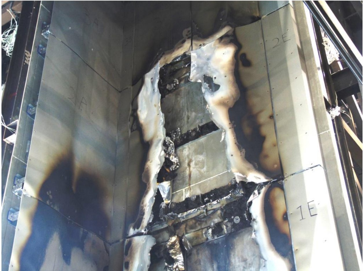
Figure 23. Damage to panels between a height of approximately 4000mm and 6000mm above the top of the combustion chamber.
