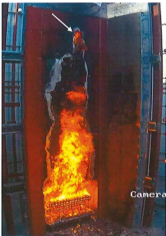
DLP C2753E/0010 Self-sustained flames on the insulation behind panels M23 & M27.
