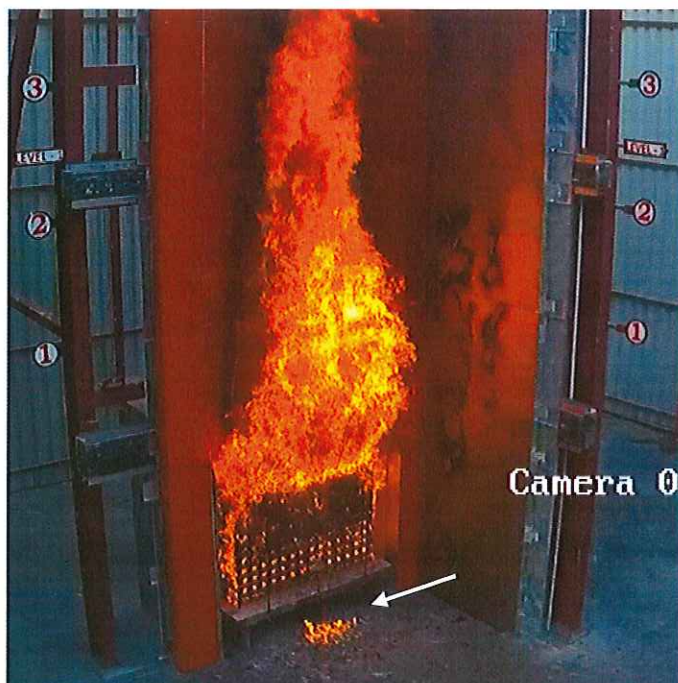
DLP C2753E/0004 Flaming debris observed on the floor.
