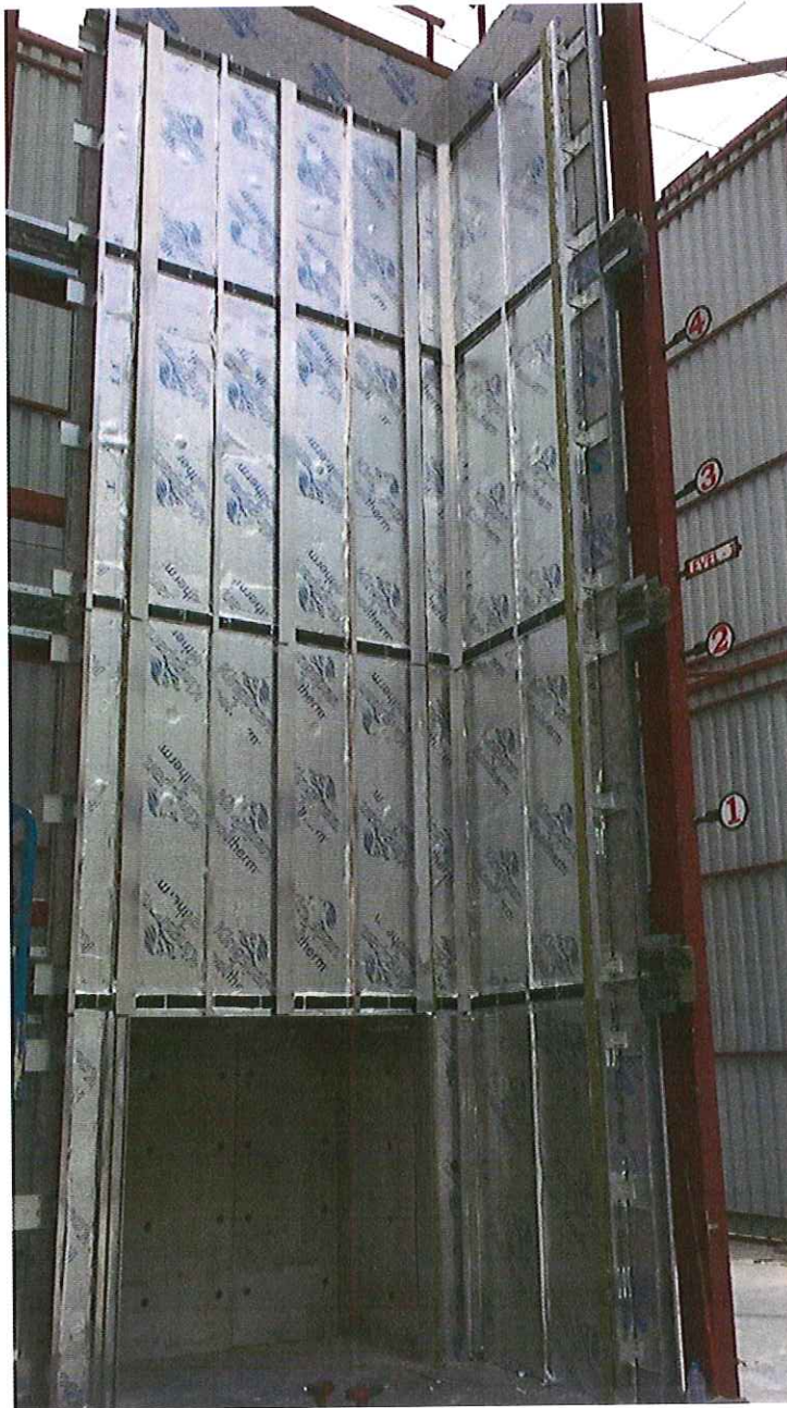
DLP C2753E/0382 Cavity barrier and Kingspan Kooltherm K15 insulation
