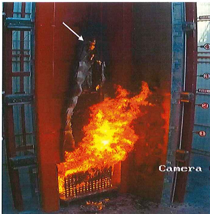
DLP C2753E/0007 Self-sustained flames behind panels M18 & M19.
