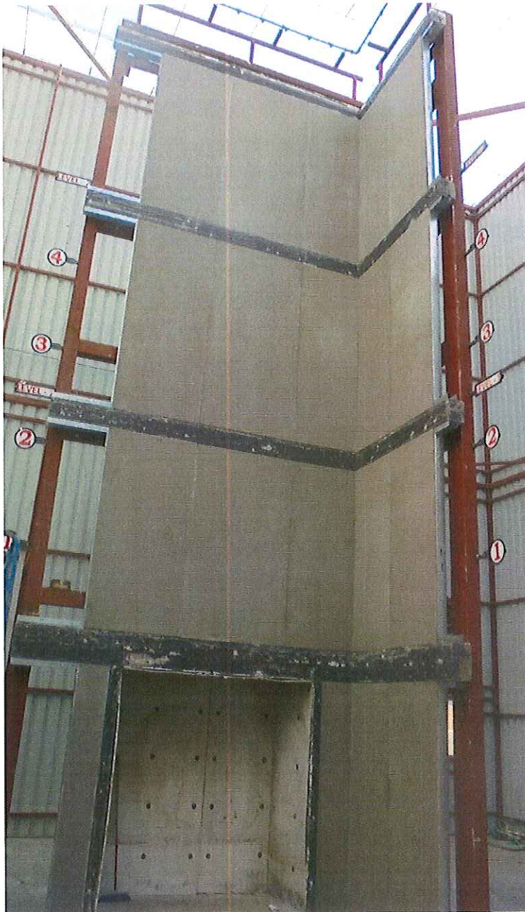
DLP C2753E/0282 12mm Versapanel cement particle board
