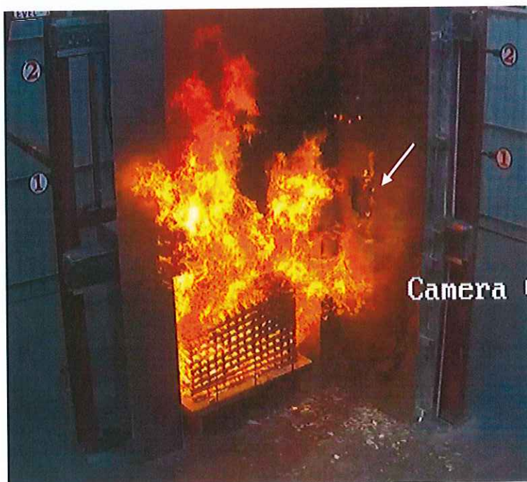
DLP C2753E/0004 Panel W2 partially melted.
