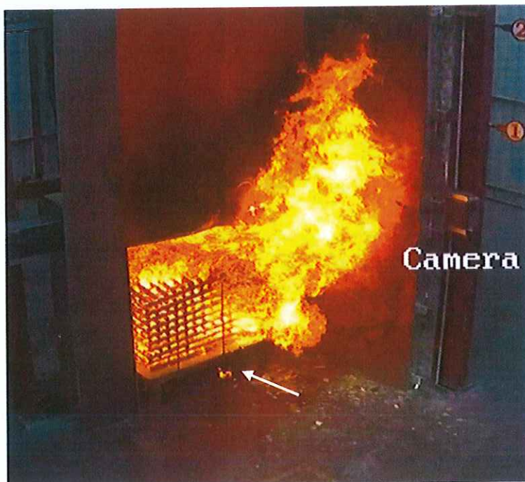
DLP C2753E/0003 Flaming debris fell off the main wall.
