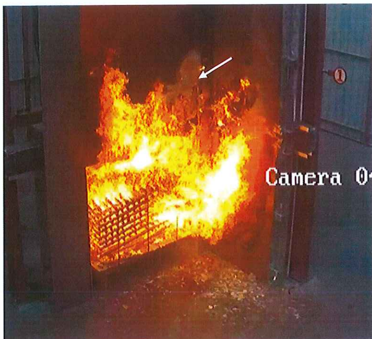
DLP C2753E/0007 Panels M5 & M6 partially melted and flames behind the panels.
