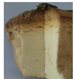
Insurer Approved PIR core sample showing extent of through-thickness charring at Suffolk Food Hall.
