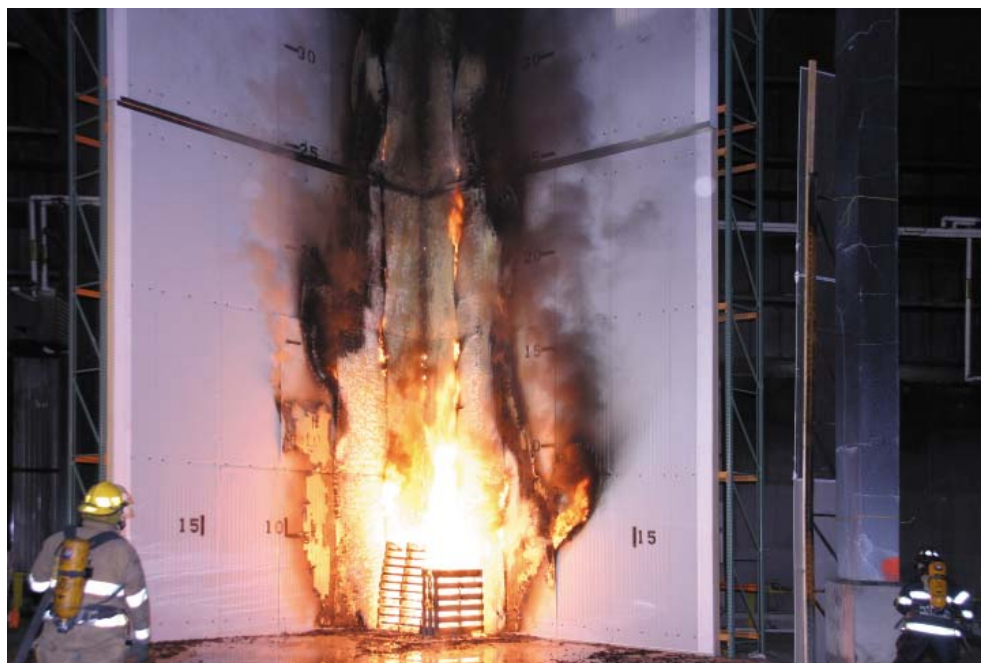
Fire is contained in the room corner – no evidence of fire propagation.
