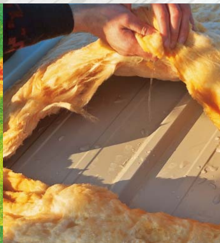
Typical example of the effect of 1% moisture ingress (by volume) on mineral fibre insulant.
