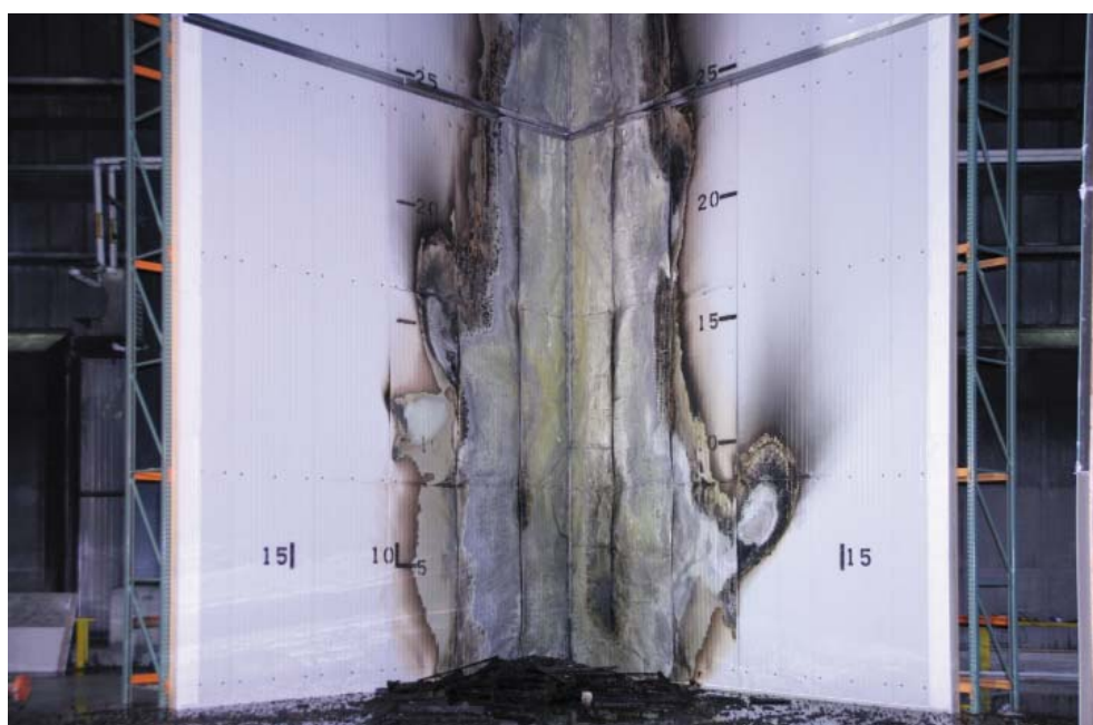
Fire is contained in the room corner – no evidence of fire propagation.
