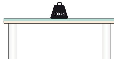
Flexural rigidity is increased by bonding the steel skin layers to the core
