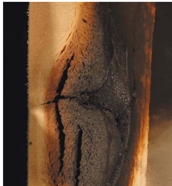
Section cut through the thickness of the panel with IPN core after 30 minutes exposure showing that the char occurs only in the area of direct flame impingement and there is no fire propagation.
