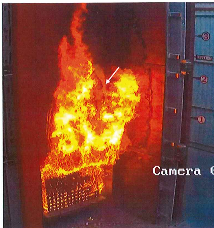
DLP C2753I/0004 Panels M4 & M5 partially melted and insulations exposed.
