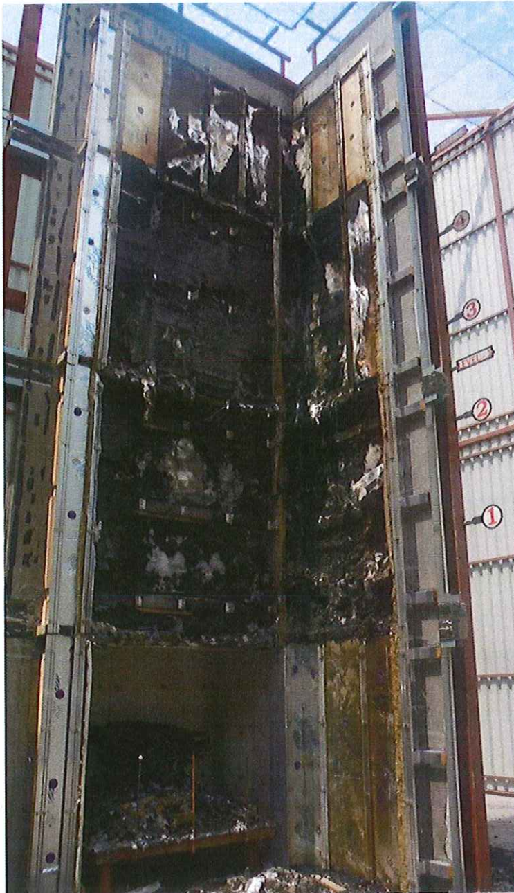
Cavity barrier, Kingspan insulation and carrier railings
