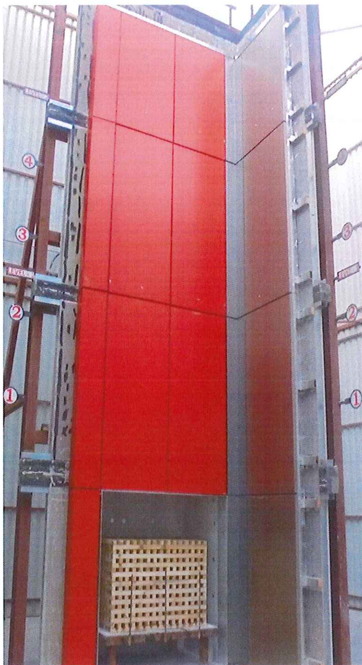
Figure 1 Photo DLP C2753I/2258 External View of the Test Sample
