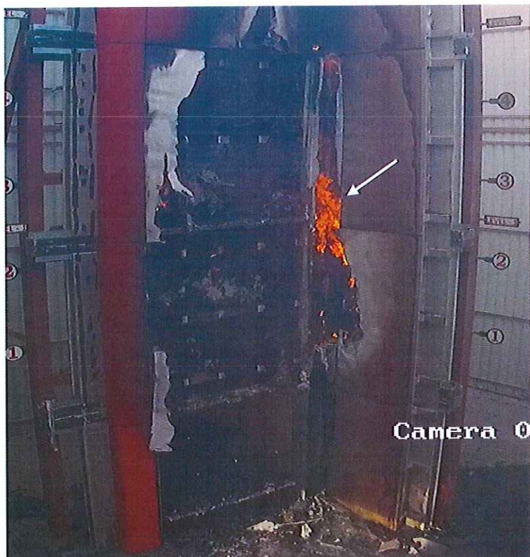
DLP C2753I/0013 Self-Sustained flames on the insulations behind the panels W3, W4 & W5.
