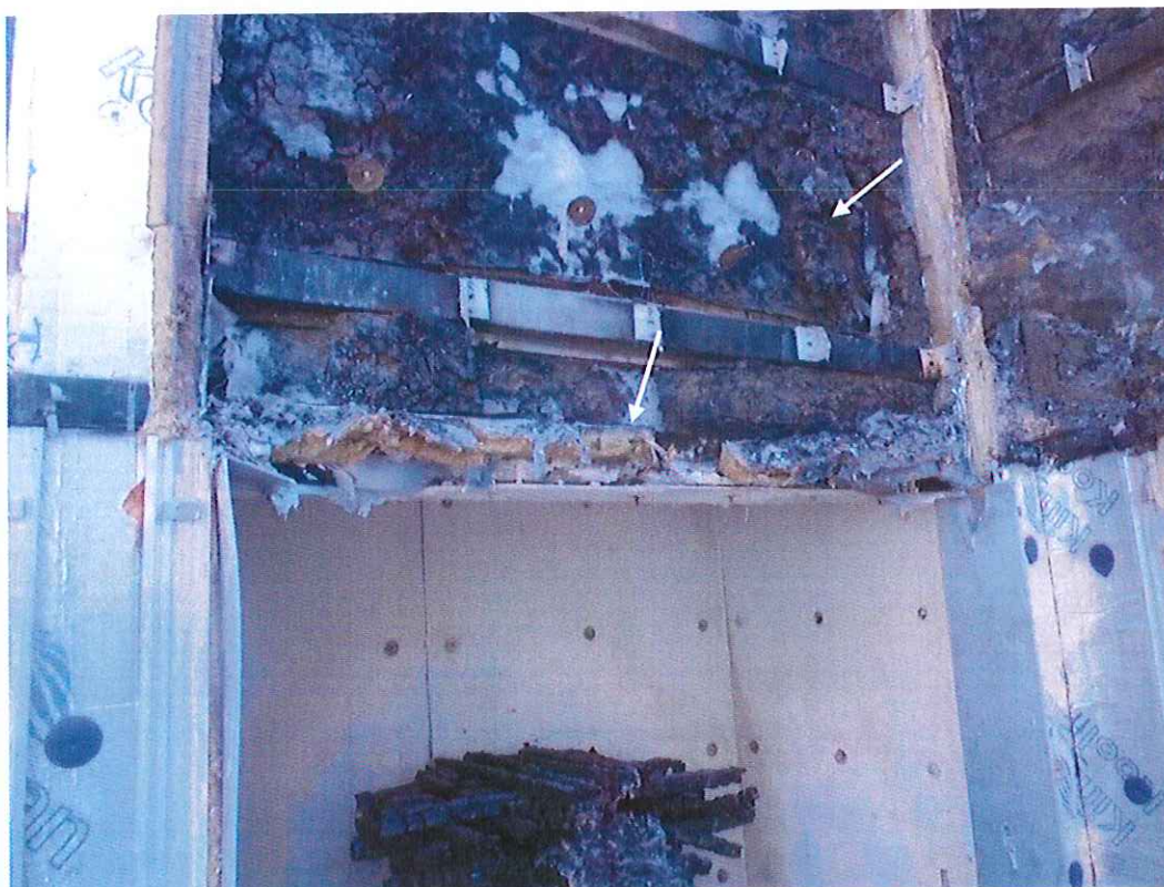
Cavity barrier and insulation above the combustion chamber
