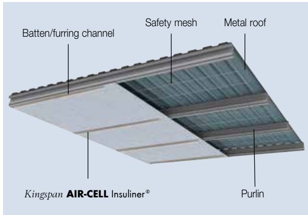
Figure 3 Warehouse metal deck roof retrofit installation
