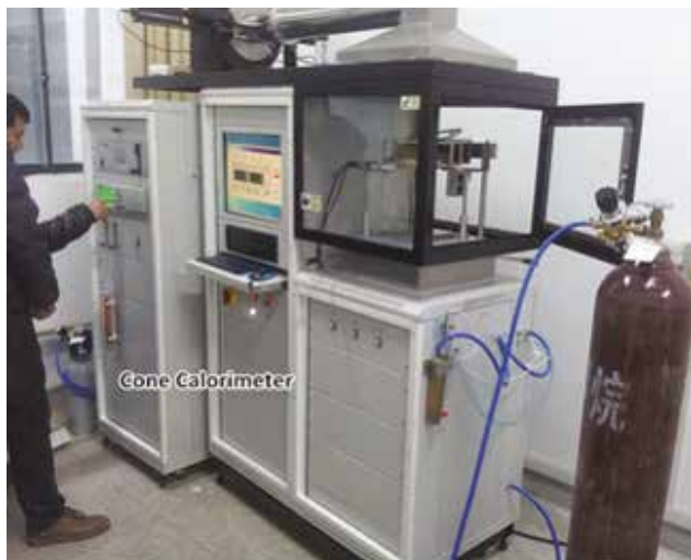
Figure 4. Cone Calorimeter Small Scale Test.
