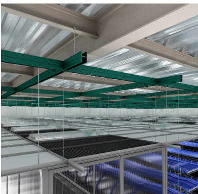
Traditional ceilings require an interstitial strut grid for hanging heavy items.
