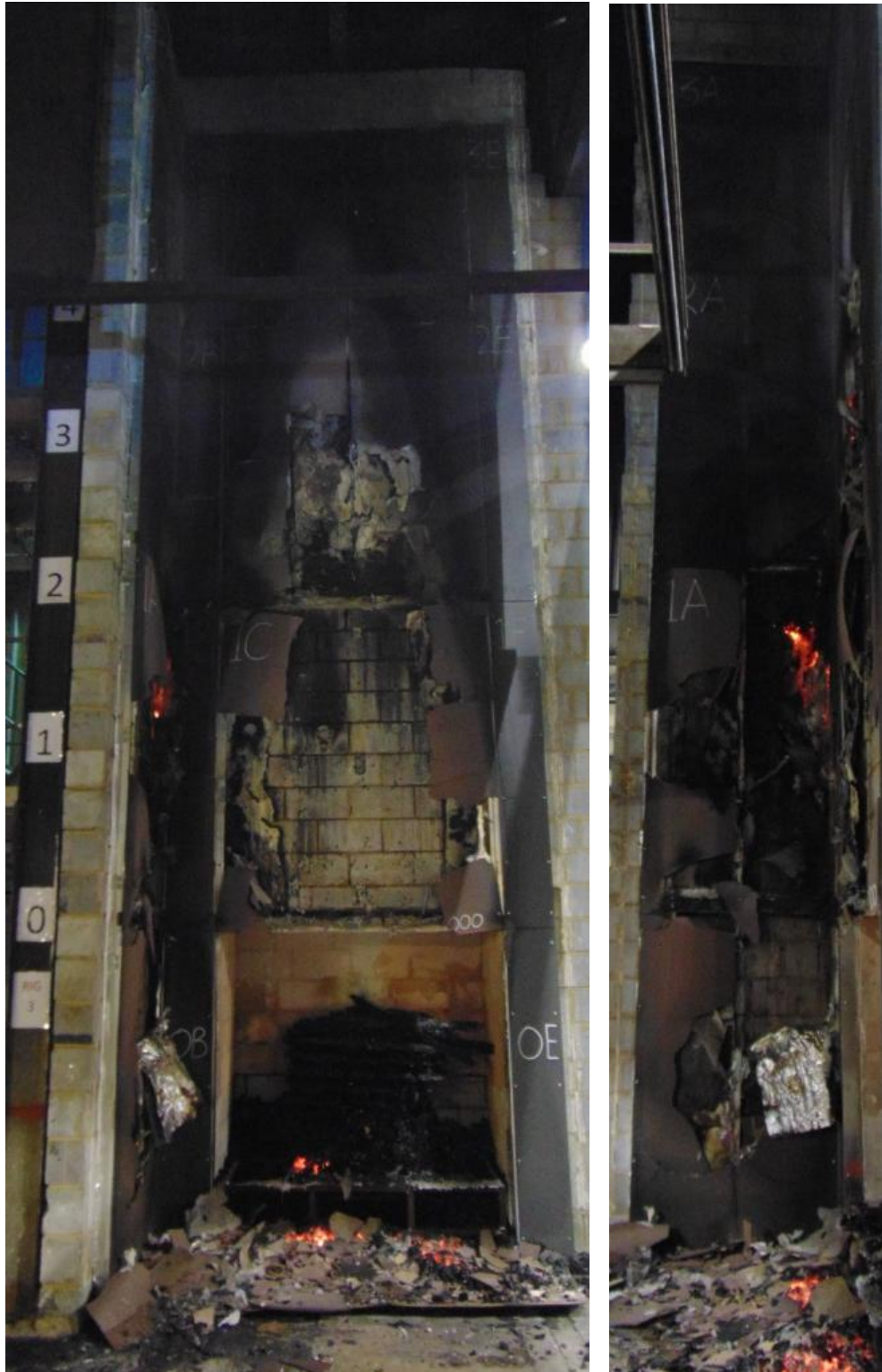
Figure 18. Full-height photograph of cladding system immediately after test.
