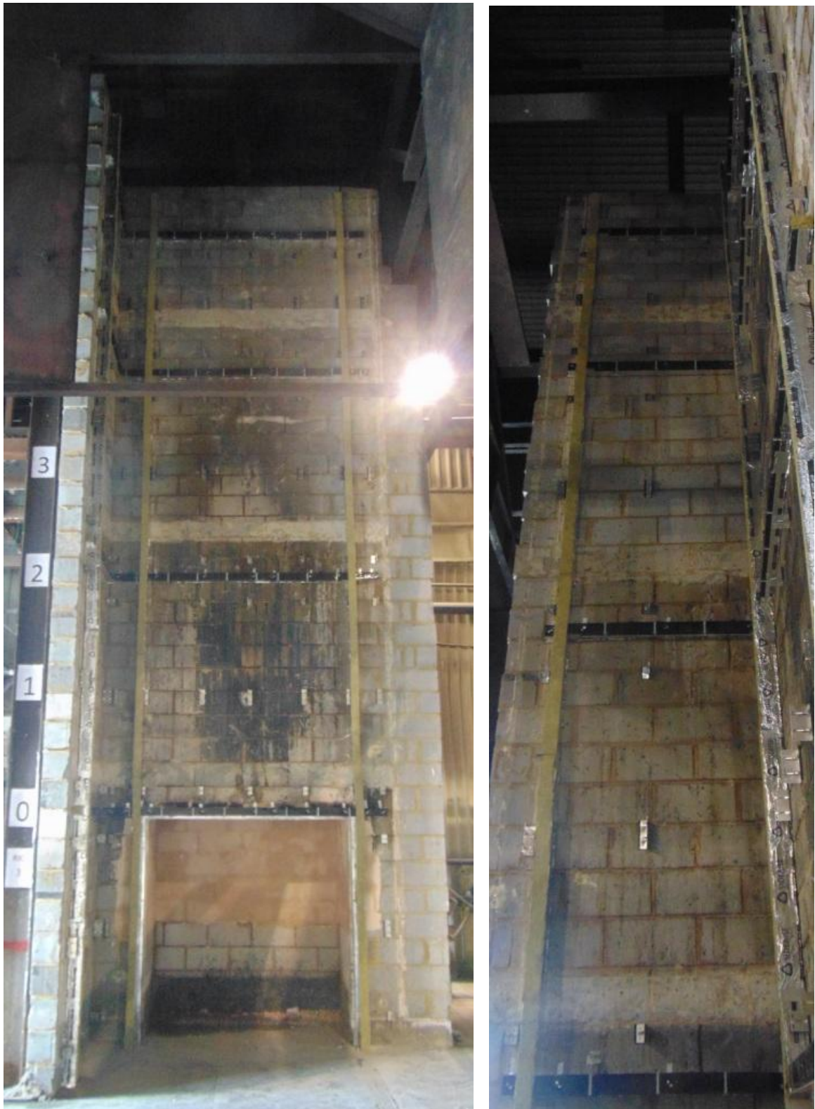
Figure 4. Installation of horizontal and vertical cavity barriers.
