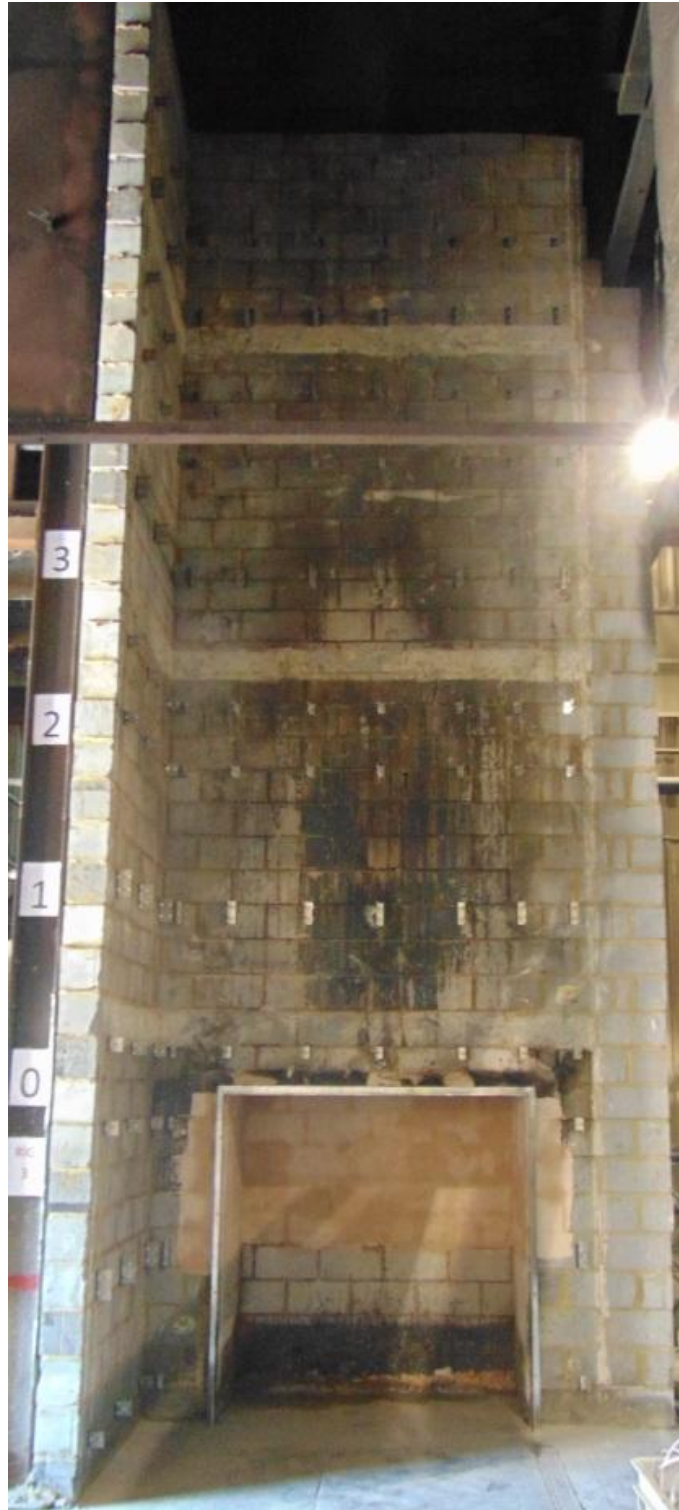
Figure 3. Installation of 'L'-shaped brackets and combustion chamber surround pod.
