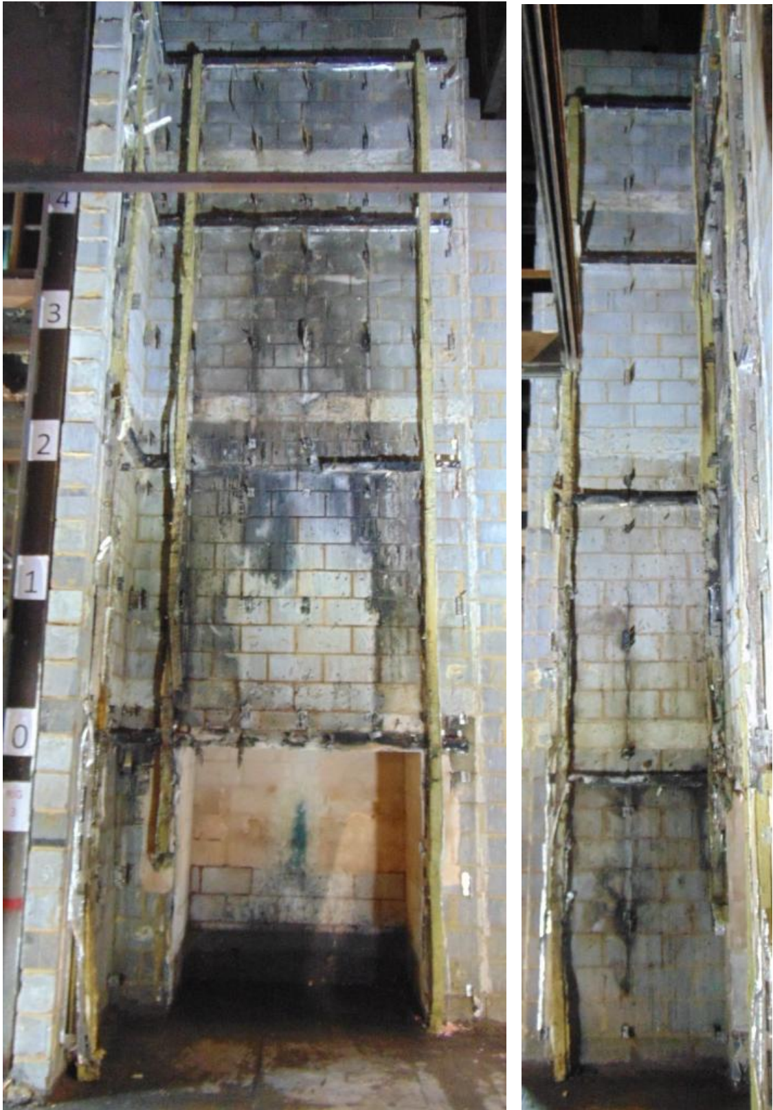
Figure 22. Post-test photograph of the horizontal and vertical cavity barriers
