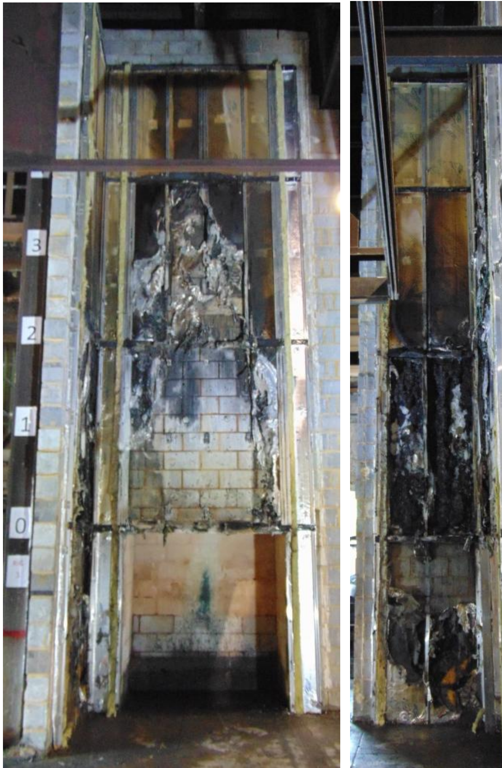
Figure 20. Post-test photograph following removal of panels.
