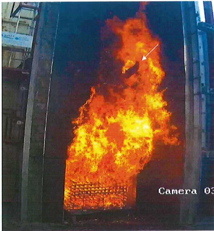
Photo 15 Flaming debris of panels M9 fell off.
