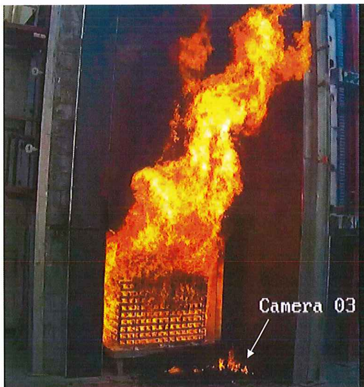
Photo 12 Flaming debris observed on the floor.
