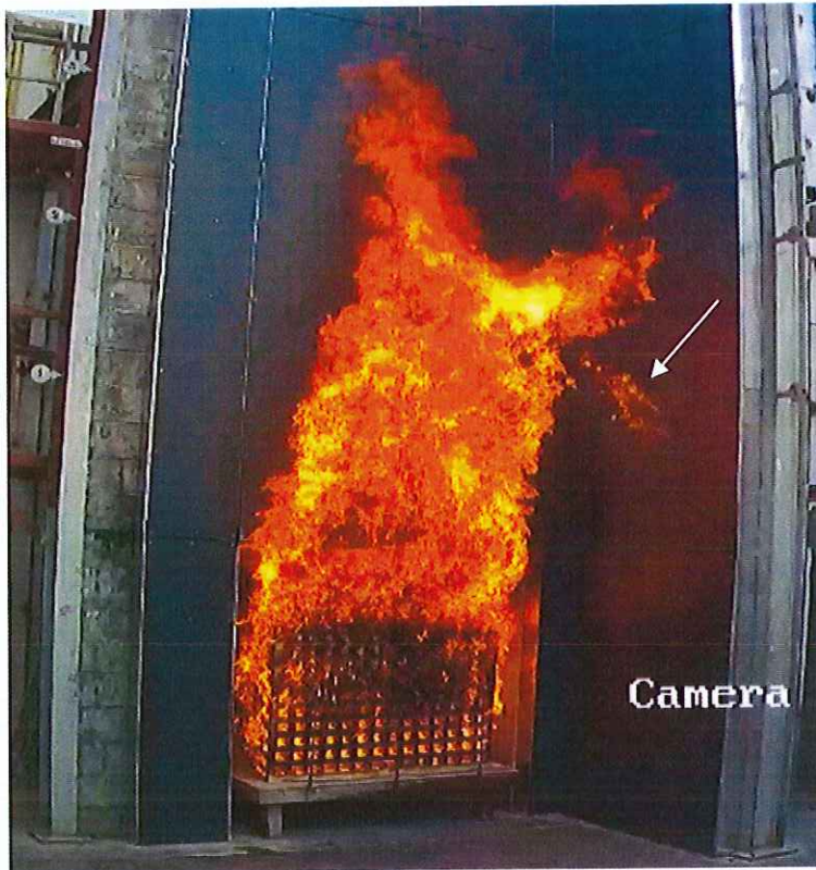
Photo 7 Flame impinged on wing wall panel W2.
