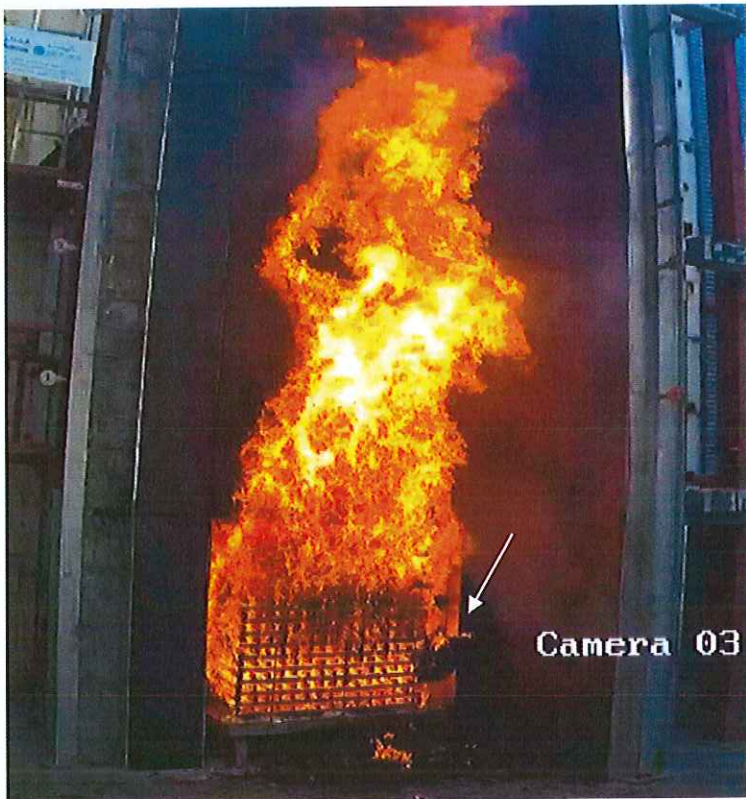
Photo 13 Flaming debris fell off the main wall.
