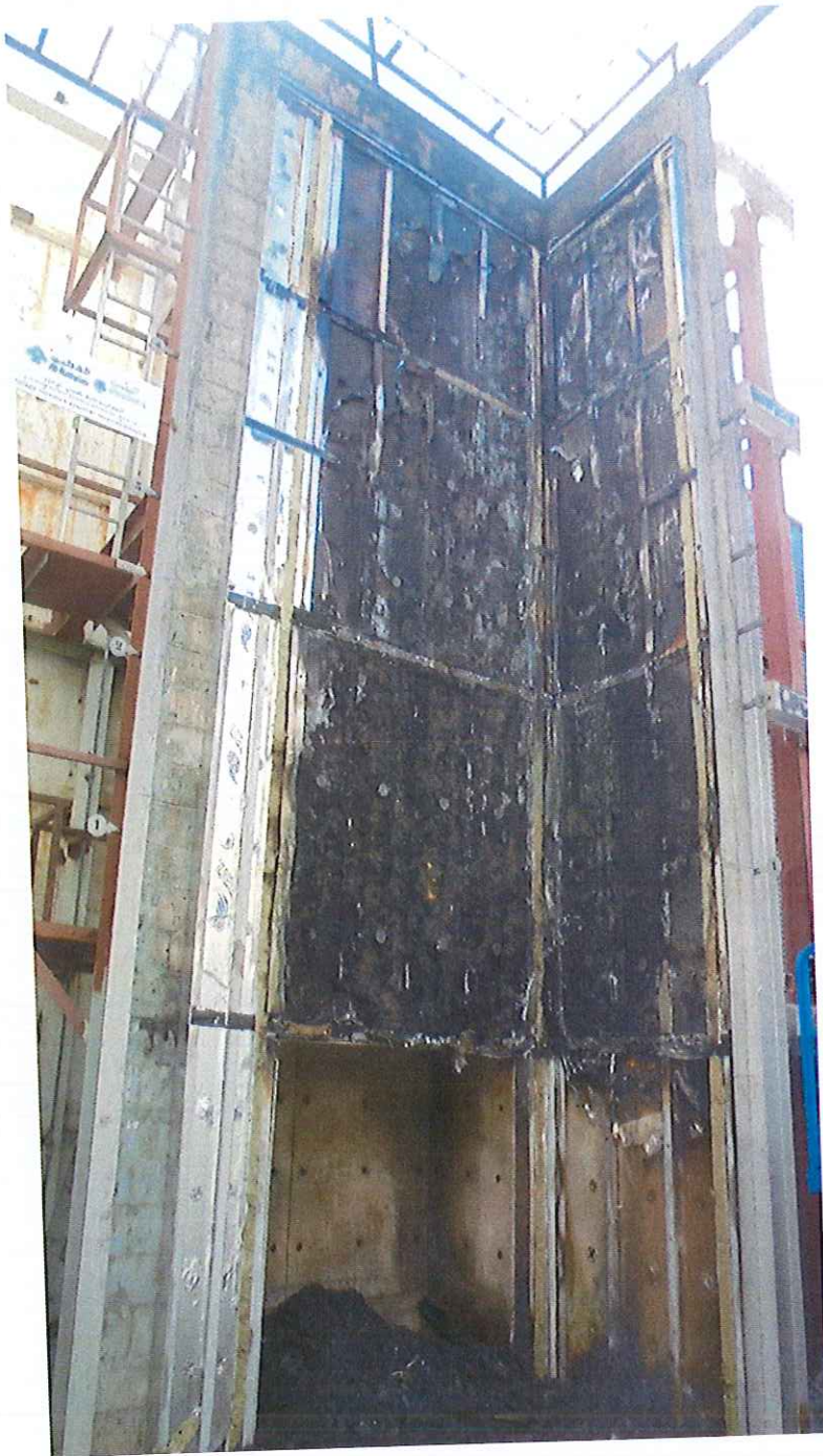
Photo 17 Cavity barrier, Kingspan Kooltherm K15 insulation and railings
