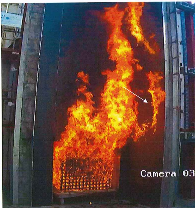
Photo 8 Self-sustained flames on surface of panel W2.
