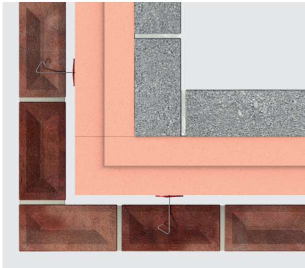
Figure 7 - Staggered Board Joint Option
