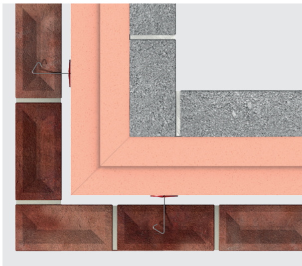
Figure 8 - Mitred Board Joint Option
