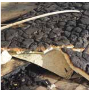
Charred PIR-insulated panel sample collected from the site
