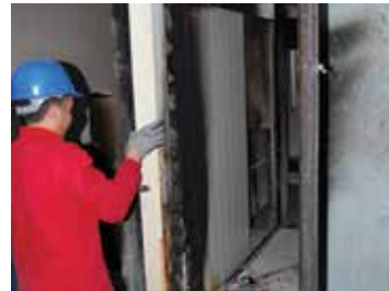
Inspection of protective char formation after test
