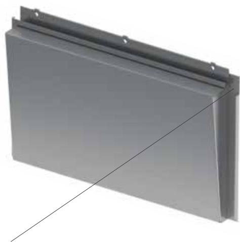
Increasing depth to one side allows a tapered variation of a standard Flat cassette; fixing system remains the same.
