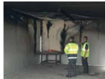
Inspection of protective char formation after test
