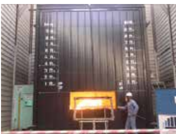
Testing of (100mm) thick Kingspan insulated metal panels
