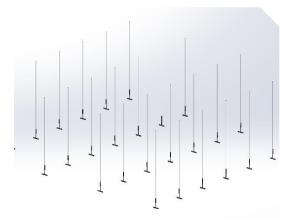
Hang turnbuckles and hanging connectors from ceiling at specified increments.
