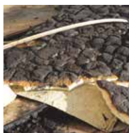
Charred PIR-insulated panel sample collected from the site
