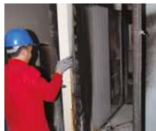
Inspection of protective char formation after test
