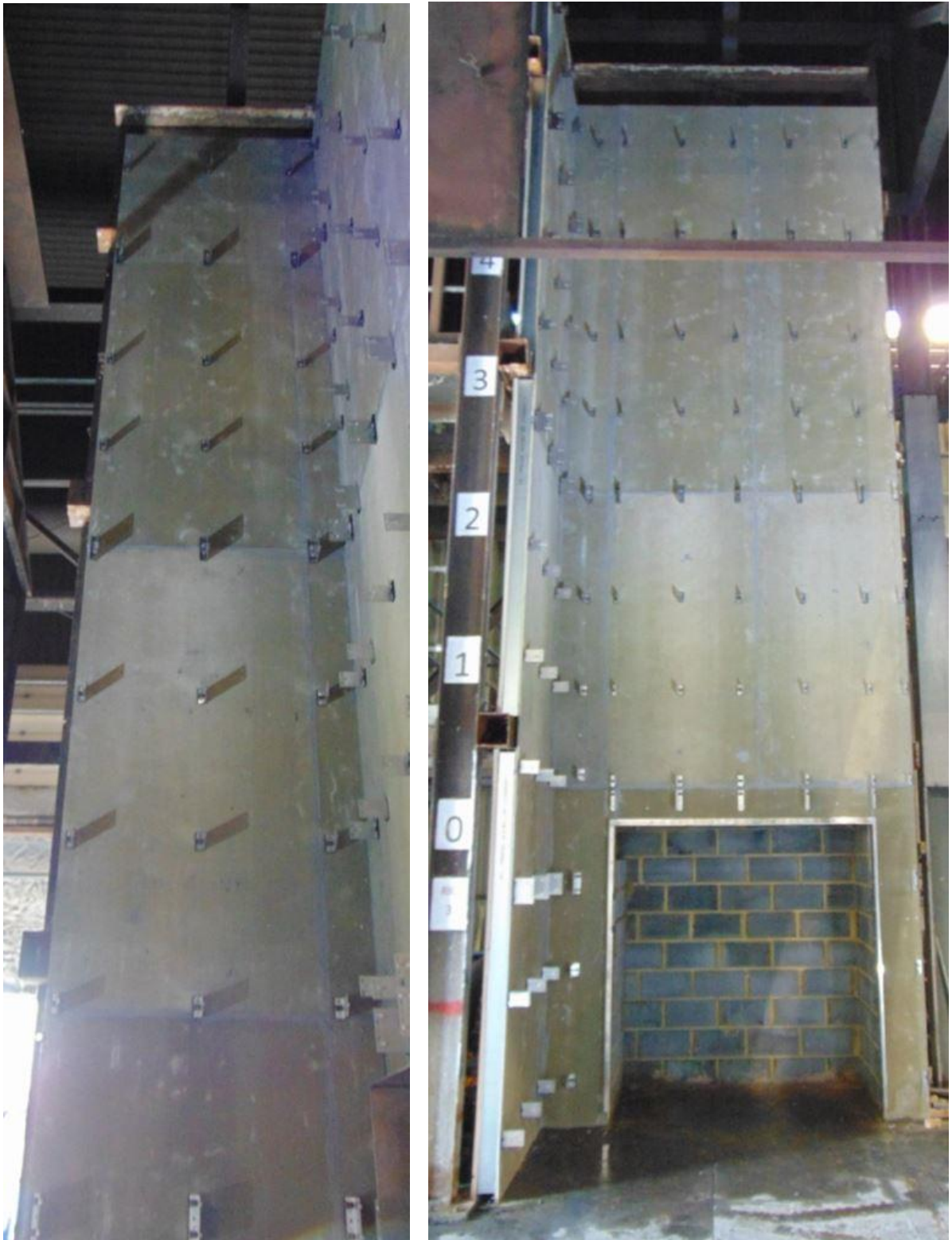
Figure 6. Installation of 'L'-shaped brackets.
