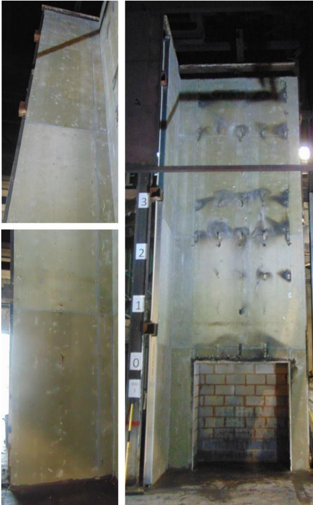
Figure 36. Post-test photograph of the cement board.
