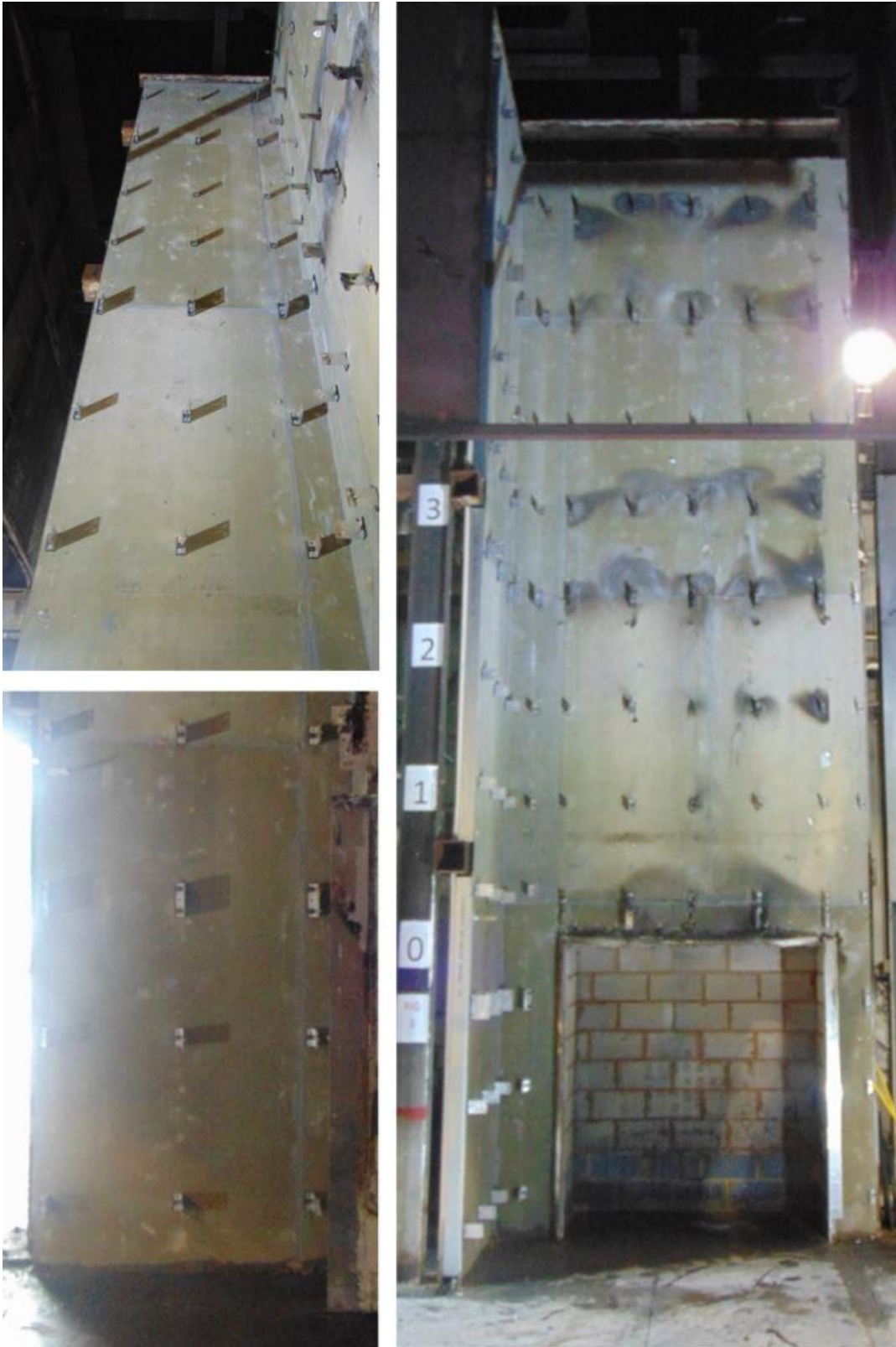
Figure 35. Post-test photograph of 'L'-brackets.
