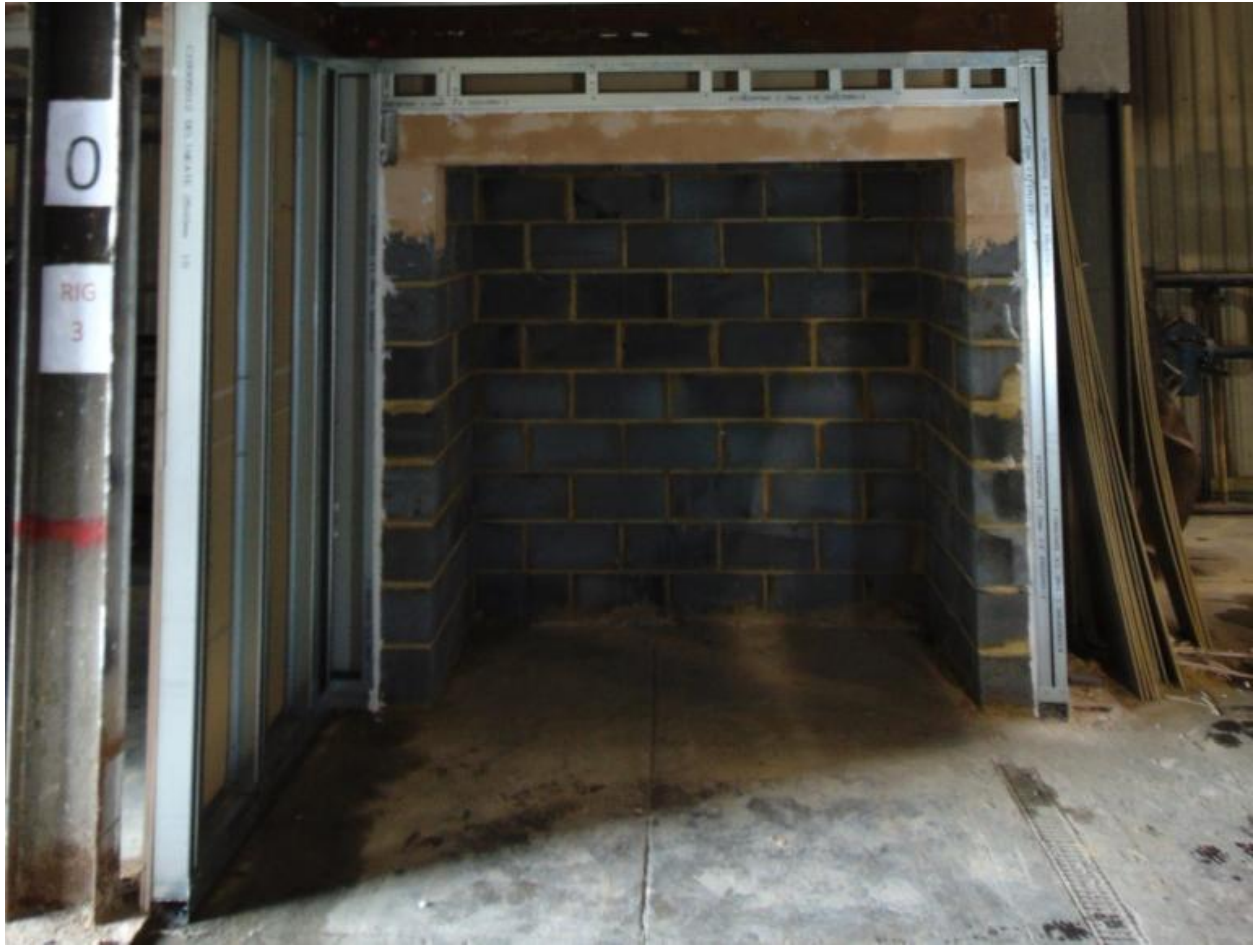
Figure 4. Sealant between SFS and combustion chamber blockwork joint.
