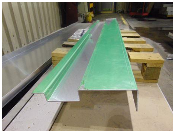
Figure 15. Profiled capping.
