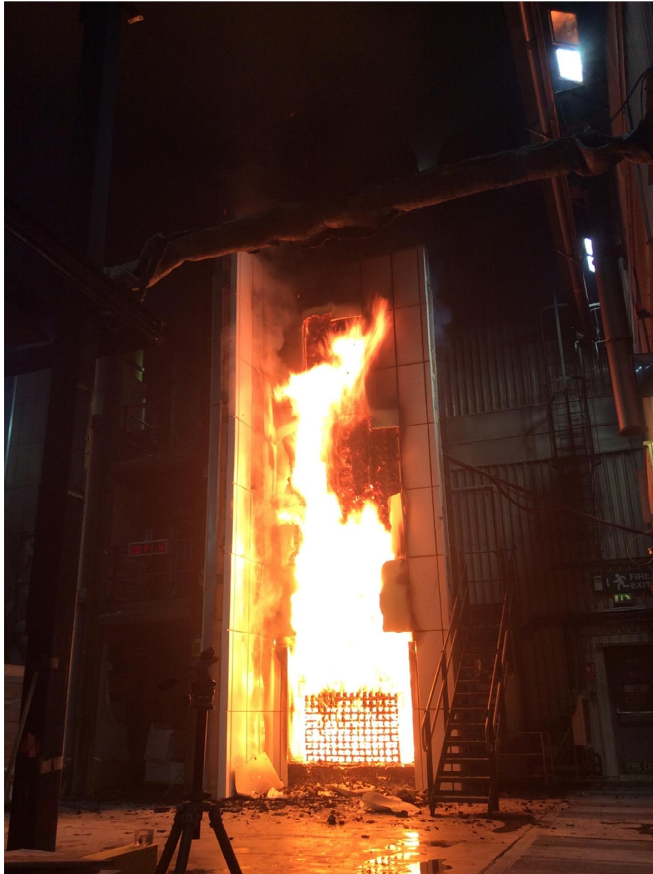
Figure 21. Increased melting/detachment of panels on main wall at approx. 6m above combustion chamber, increased debris (00:21:12 from ignition)
