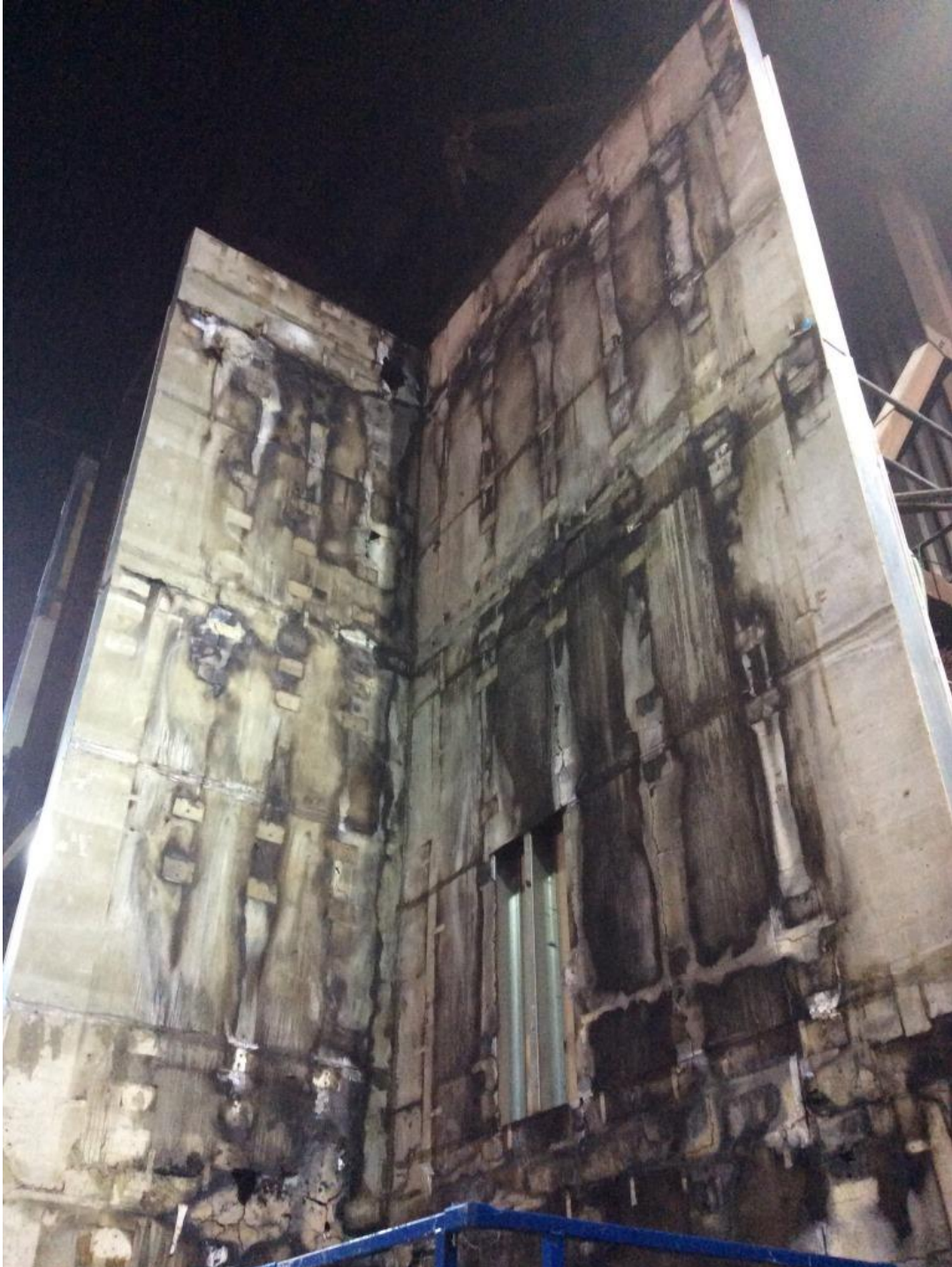
Figure 41. Post-test photograph of sheathing board layer.
