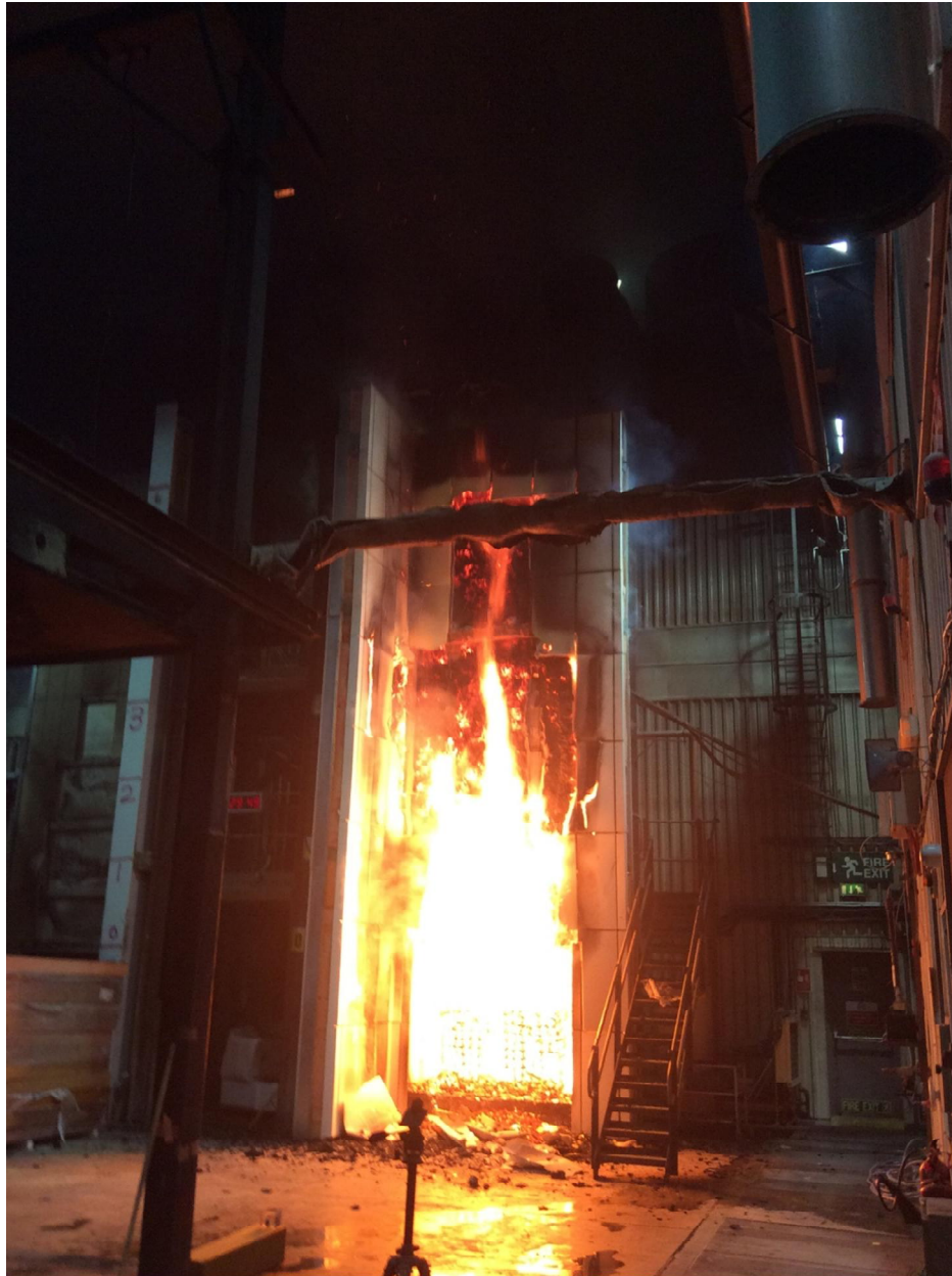
Figure 24. Flaming from top row main wall panel to top of test specimen (00:29:49 from ignition)
