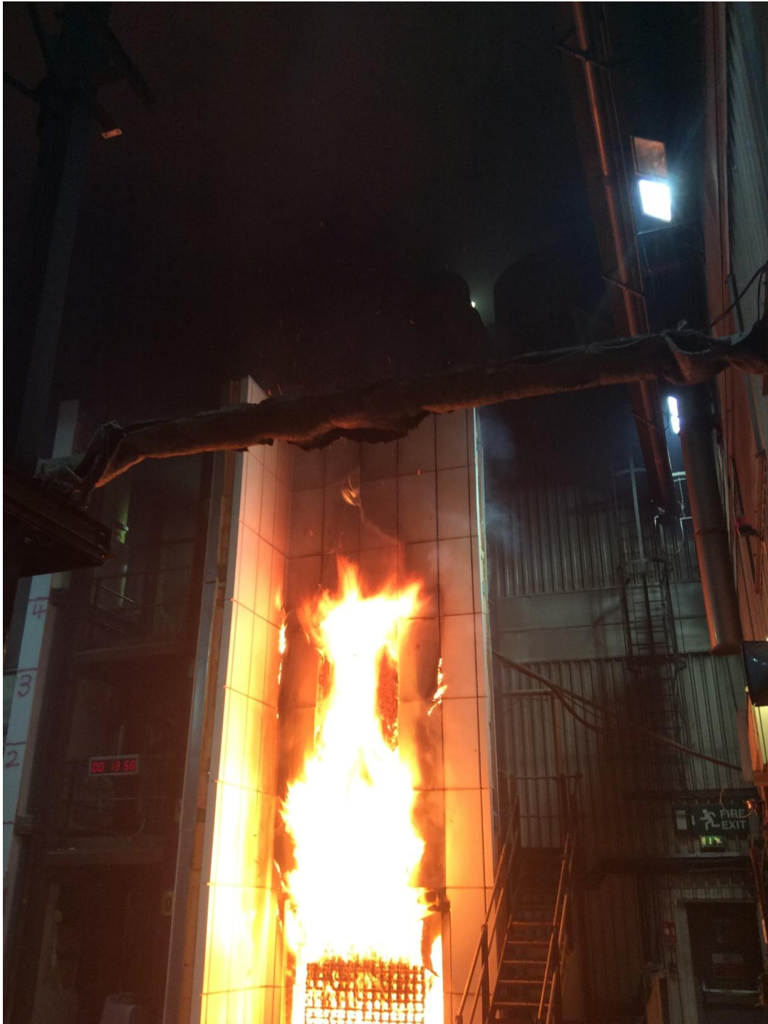
Figure 17. Main wall panels melted/detached to approx. 3.5m above combustion chamber, flaming at main-wing wall junction (00:13:56 from ignition)
