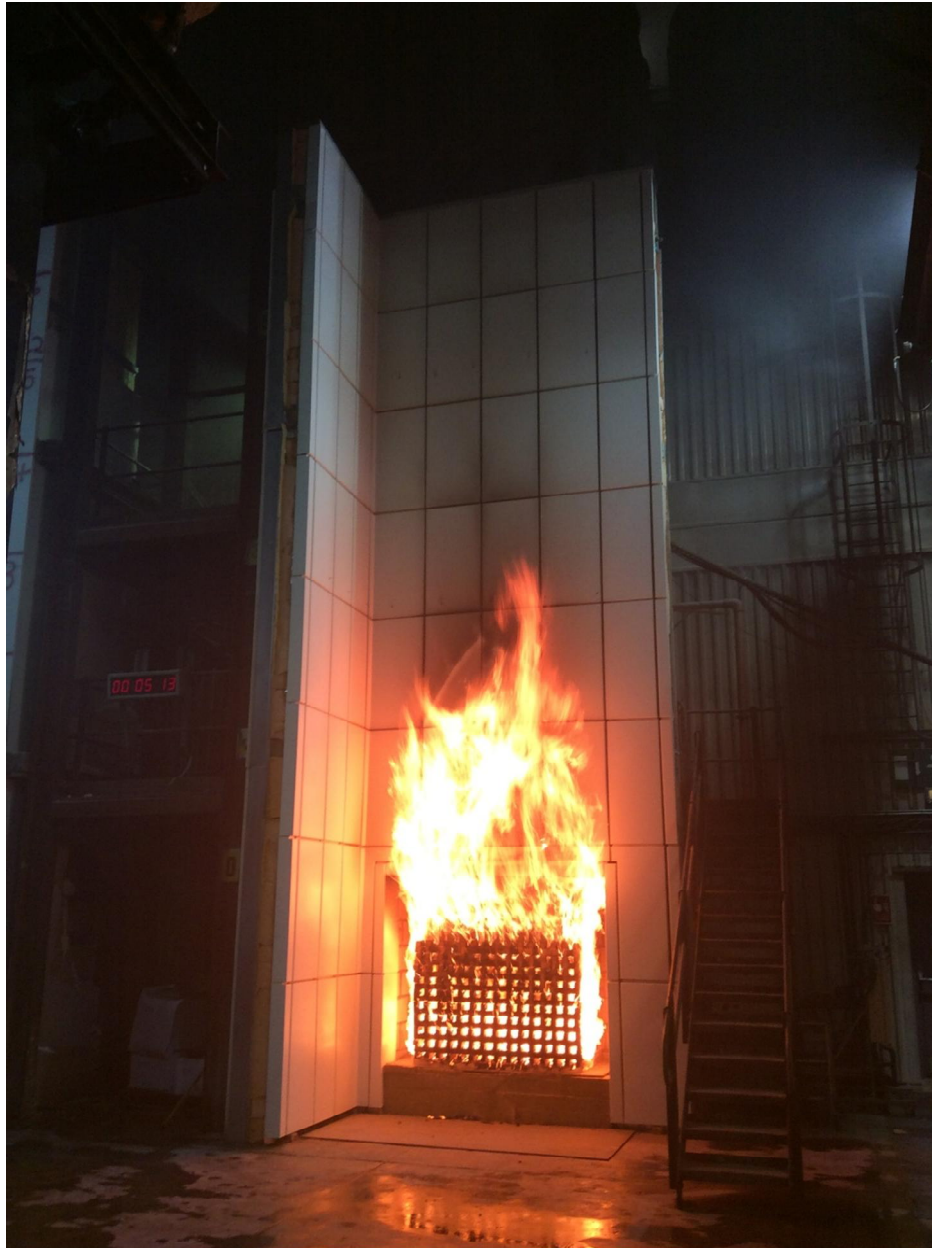
Figure 15. Flame tips to approx. 2.5m above combustion chamber (00:05:13 from ignition)
