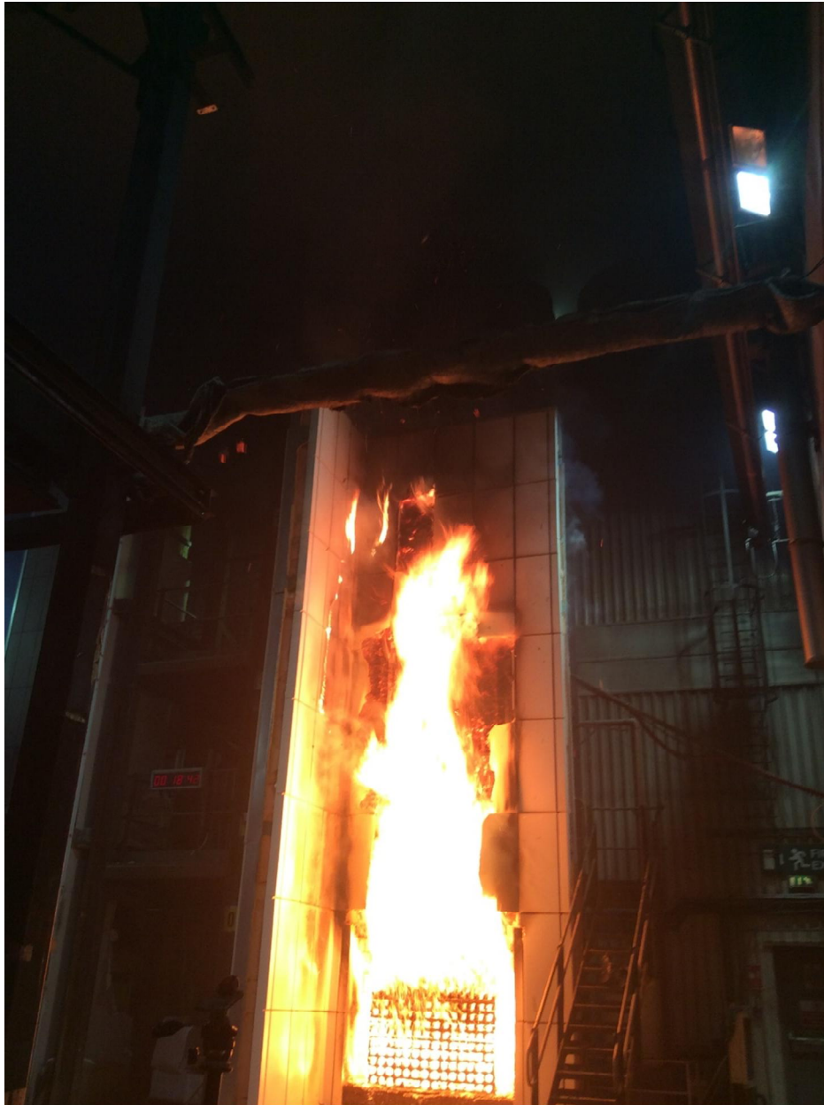
Figure 19. Increased melting/detachment of main wall panels up to approx. 6m above combustion chamber, flaming from main and wing wall at this height (00:18:42 from ignition)
