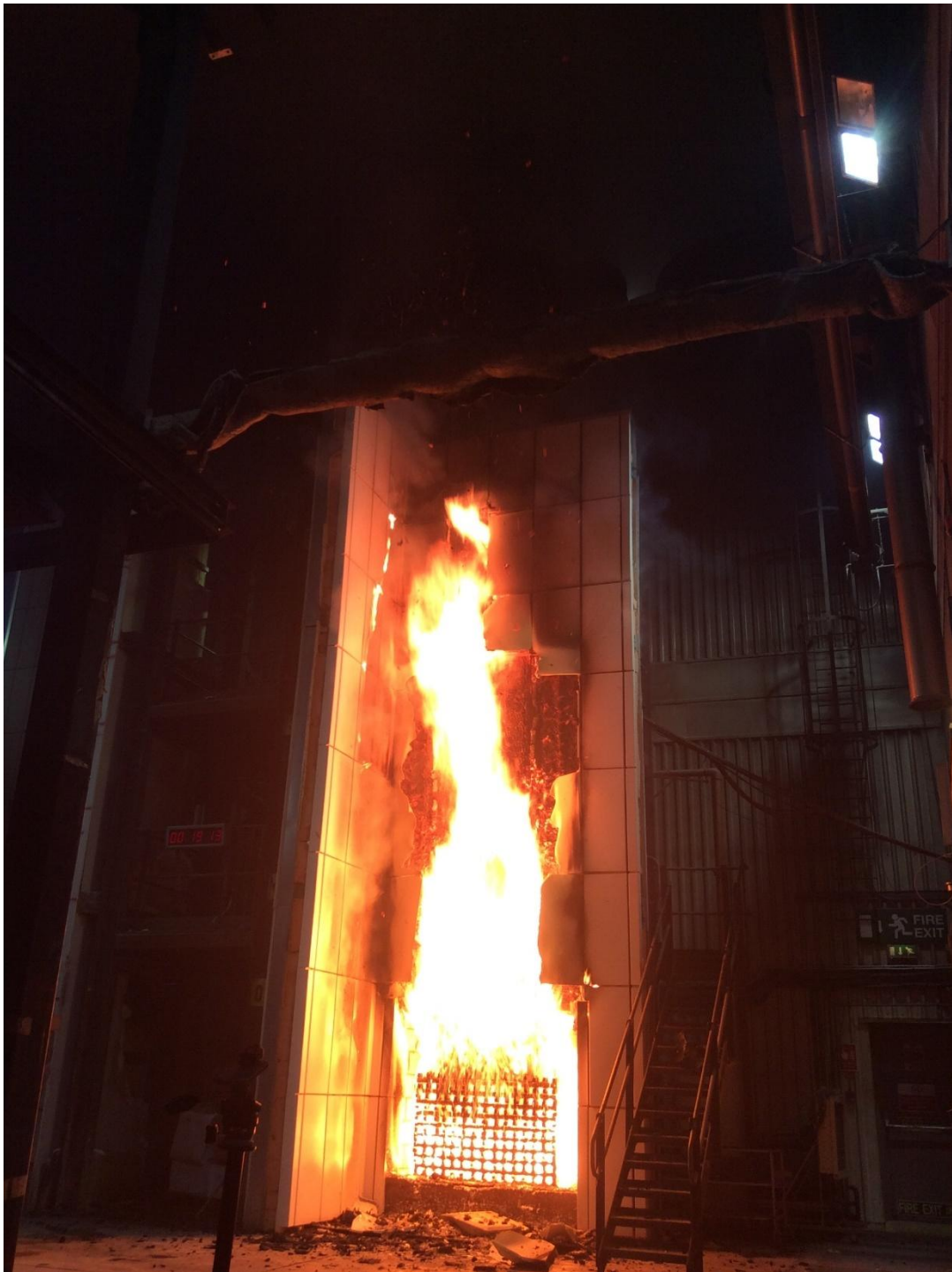
Figure 20. Increased flaming from main wall at approx. 6m above combustion chamber, increased debris (00:19:13 from ignition)
