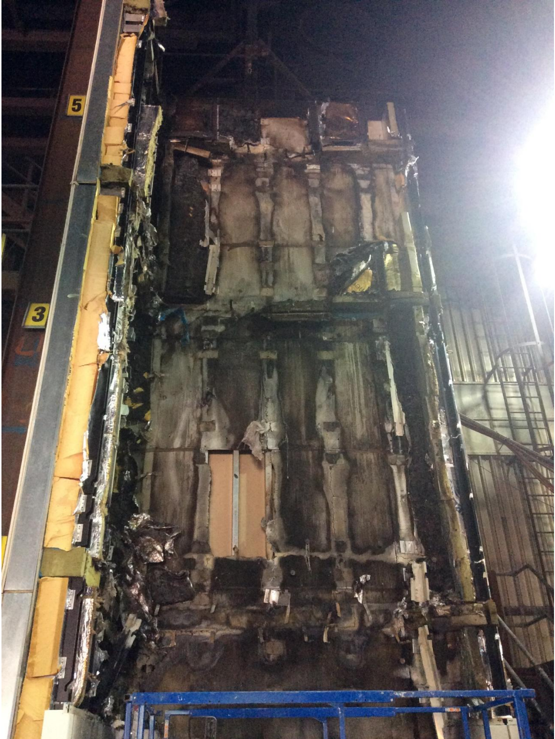
Figure 39. Post-test photograph of main wall following panels removal.
