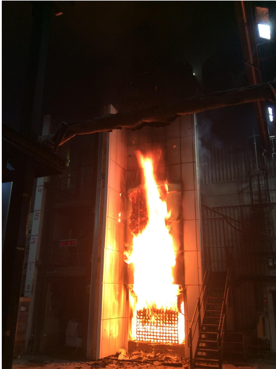
Figure 18. Increased melting/detachment of main wall panels, flaming from wing wall at approx. 3.5m above combustion chamber (00:16:34 from ignition)
