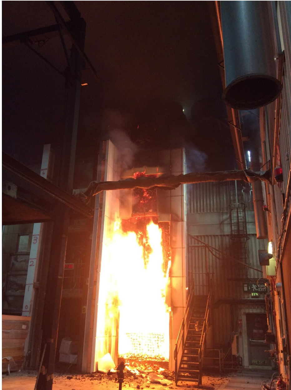
Figure 23. Melting of panels and insulation smouldering to top row of main wall panels, increased flaming from wing wall (00:27:08 from ignition)
