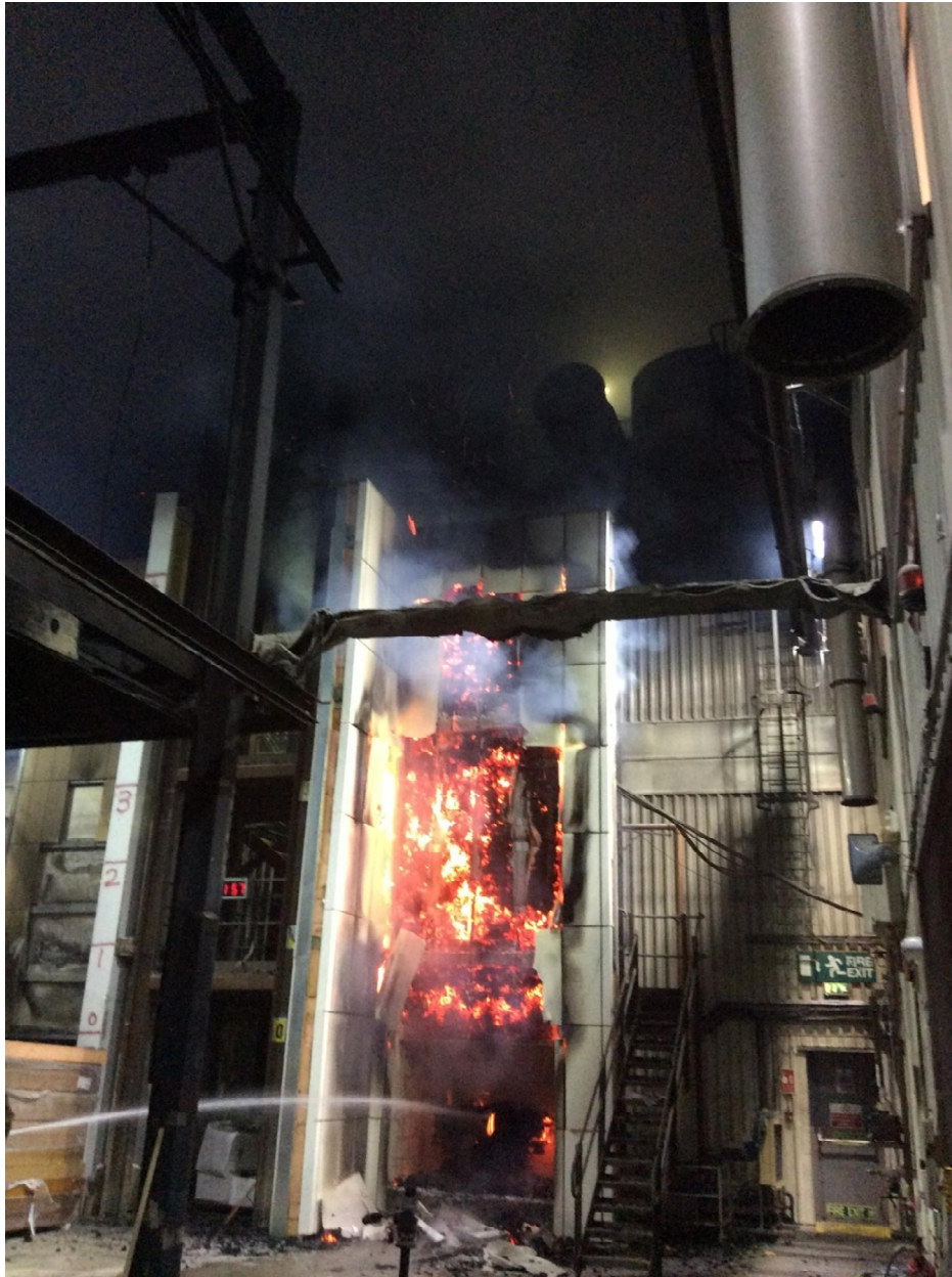
Figure 25. Crib extinguished at 30 minutes from ignition, flaming from top of test specimen (approx. 32mins)
