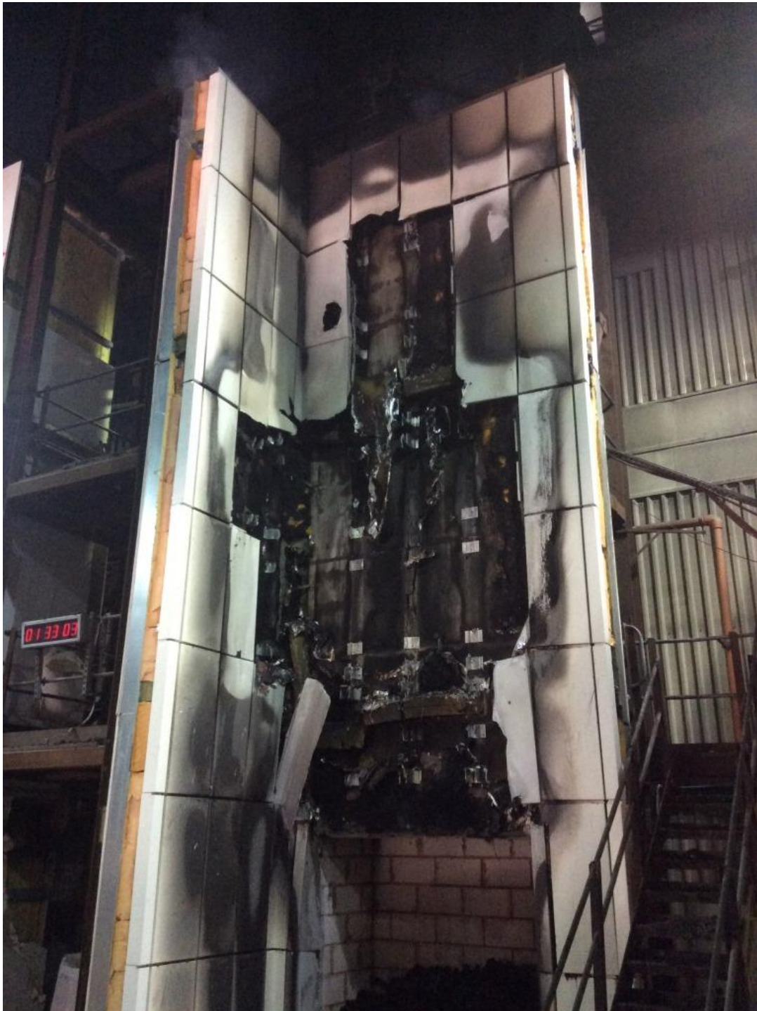
Figure 38. Full-height photograph of cladding system following post-test dousing.
