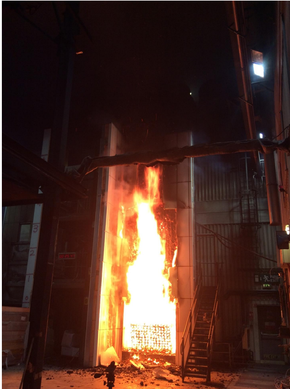
Figure 22. Melting of wing wall panel at approx. 3m above combustion chamber (00:25:47 from ignition)
