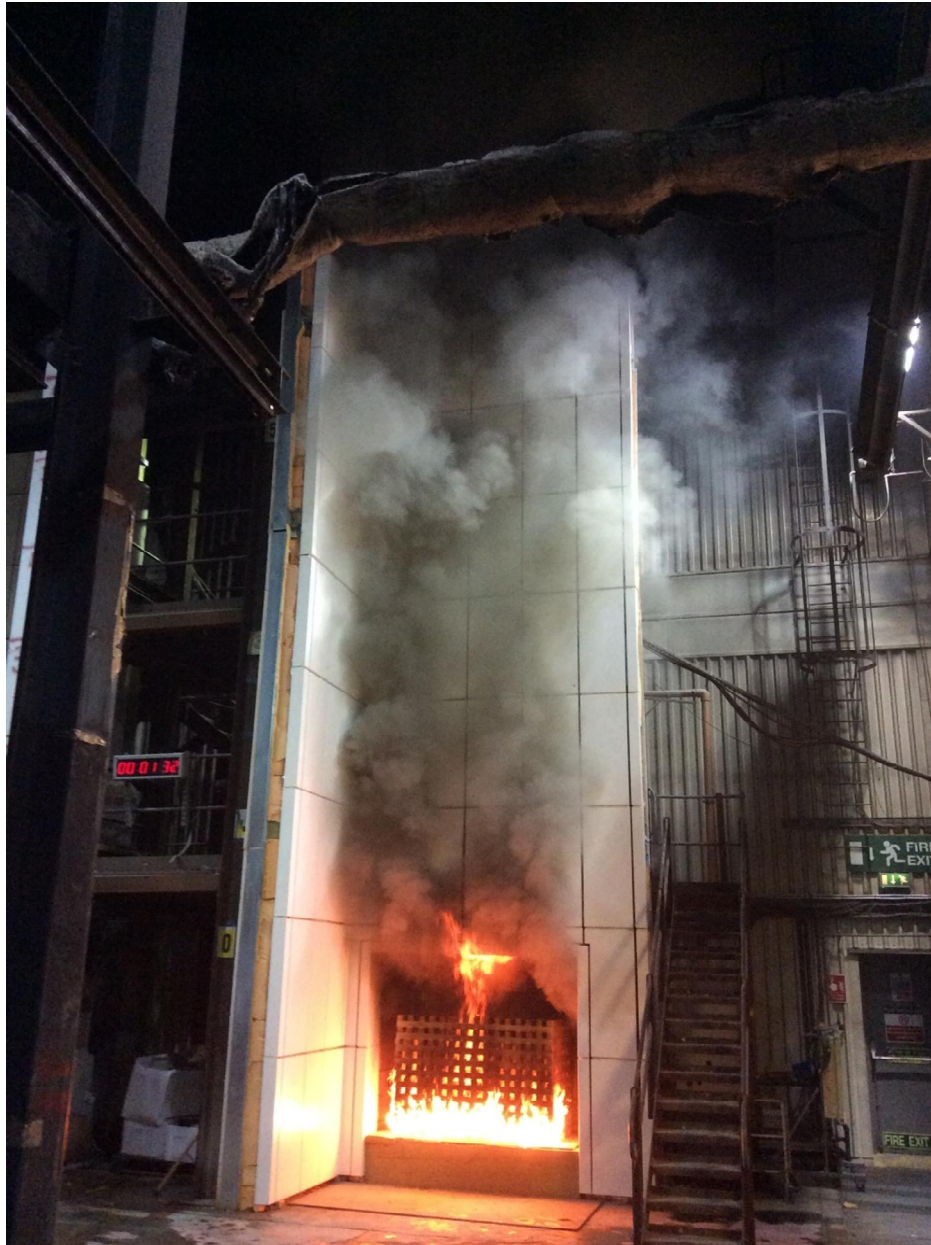
Figure 14. Flames escaping combustion chamber (00:01:32 from ignition)
