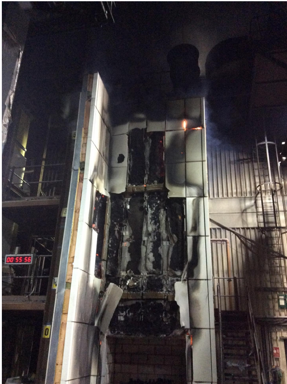
Figure 29. Significant reduction in flaming except at outside edge of main wall, 6m above combustion chamber (00:55:56)
