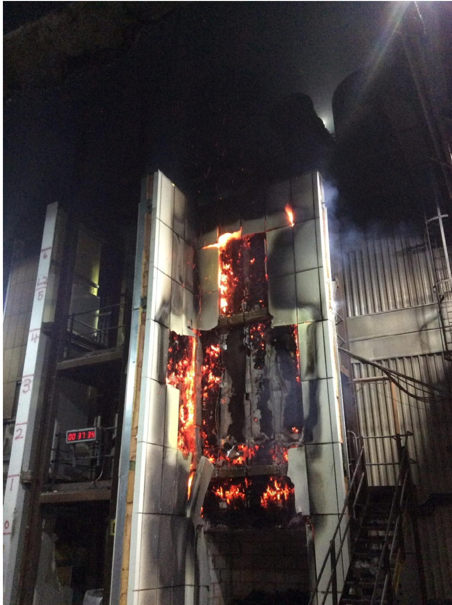
Figure 27. Increased flaming from behind main wall panels at approx. 6m above combustion chamber (00:37:39)
