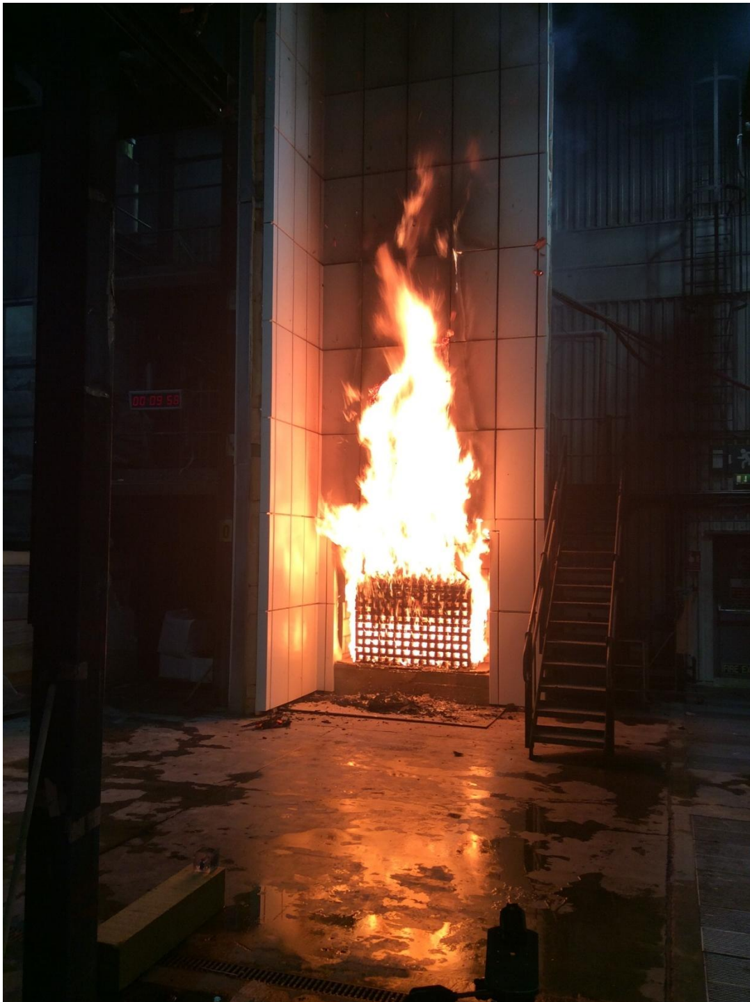
Figure 16. Main wall panels melted to approx. 2m above chamber, falling debris (00:09:56 from ignition)
