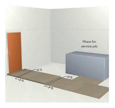
Heavy loads, such as blowers etc. applied during installation, have to be checked. The panels should always be protected during the installation phase using load-distributing plywood boards. Such protection should also be used for stepladders etc. point loads.
