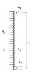
t = steel sheet thickness L<sub>s</sub>= support width T<sub>2</sub> - T<sub>1</sub> = 55 °C
