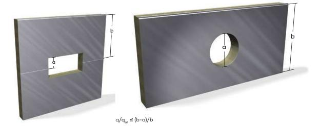
If the degree of cut-out exceeds the ratio  $q/q_{all}$ , the load is either to be transferred to adjacent panels in accordance with figure 14 or, if this is not possible, to be directed on the loadbearing frame by auxiliary structures. See also dimensioning example in the following section.
