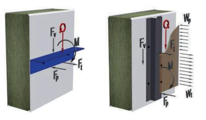
Shear force F<sub>v</sub> Tensile force F<sub>t</sub> Pressure force F<sub>p</sub>
