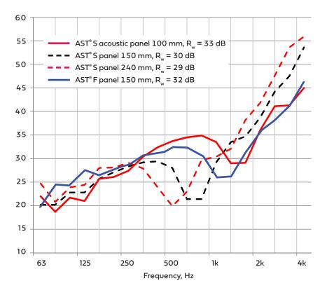
Table 17. Weighted sound reduction of PPS panels at various noise spectra, panel type  $\mathsf{AST}^*\,\mathsf{S}.$
