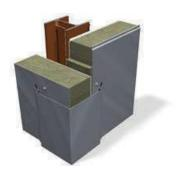
$\Psi$  = 0.02 W/m for a 100 mm panel and 0.008 W/m for a 200 mm panel
