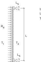
t = steel sheet thickness  $L_s$  = support width  $T_2$  -  $T_1$  = 55 °C
