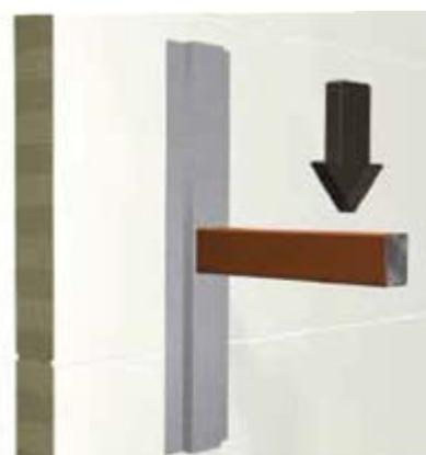
With increasing loads, the number of required fixings increases linearly, e.g. Load = 40 kg, the number of fixings is 2 x the number given in the table above. Load = 60 kg, the number of fixings is 3 x the number given in the table above. Note! In the shaded area of the table, always use 2 fixings at the top end of the load-bearing unit.
