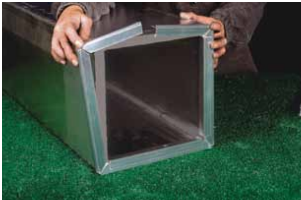
Figure 10.3 Bending the Aluminium Grip External Profile
