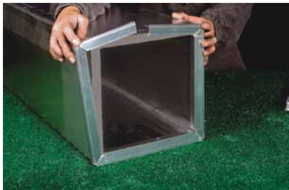
Figure 10.3 Bending the Aluminium Grip External Profile
