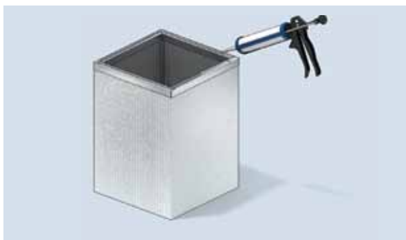
Figure 10.18 Application of Silicone Sealant
