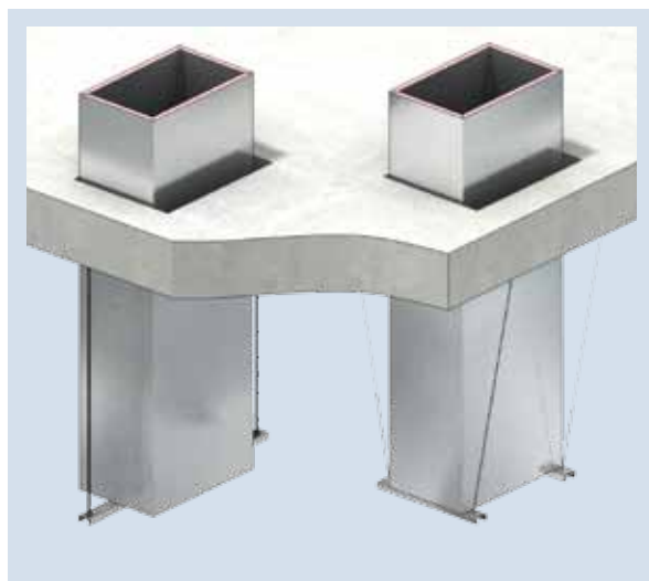
Figure 15.1 Conventional Hangers & Supports for Vertical Ductwork
