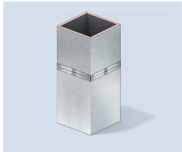
Figure 10.19 Fitting Tiger Clips
