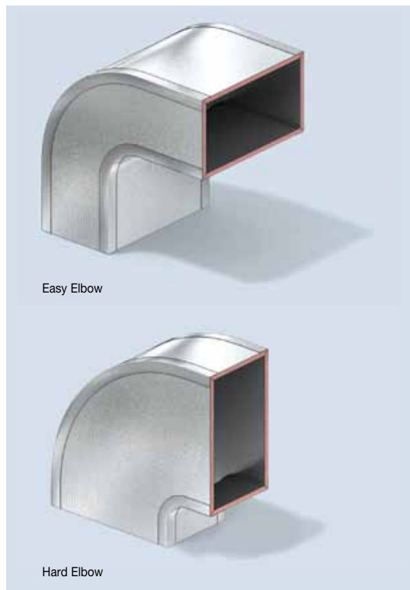
Figure 4.2 Hard or Easy Elbow
