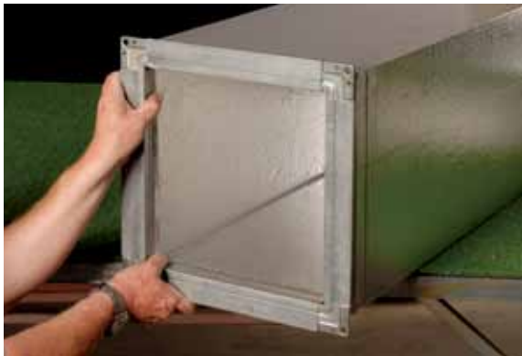
Figure 10.11 Fitting the 4-bolt Profile
