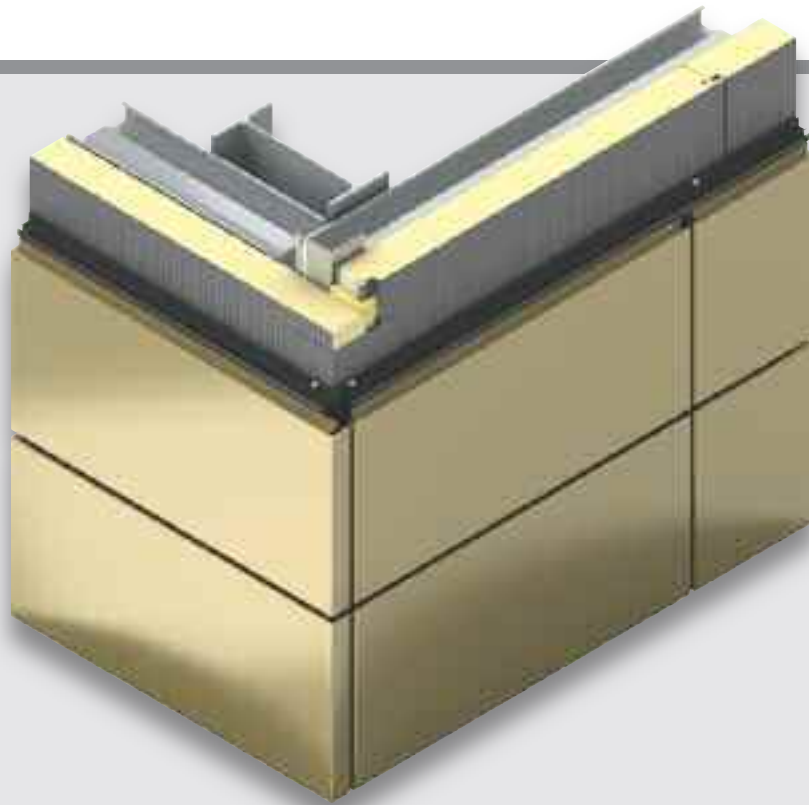
External Corner Detail Vertical Application
