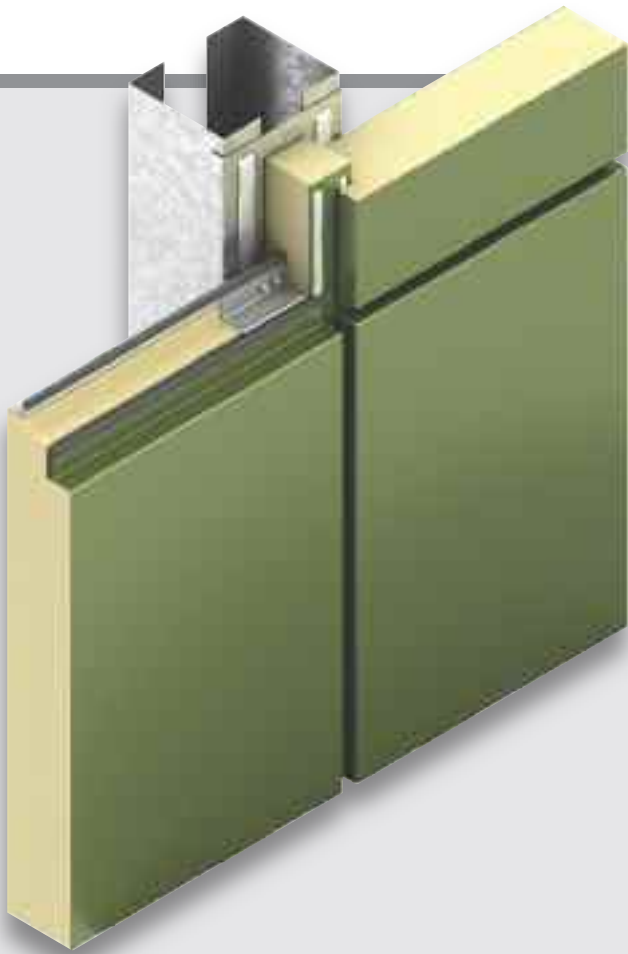
End Lap Detail - C4 Horizontal Application
