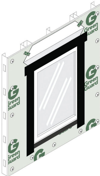
Figure 9 Installation of Window and Jamb and Head Flashings
