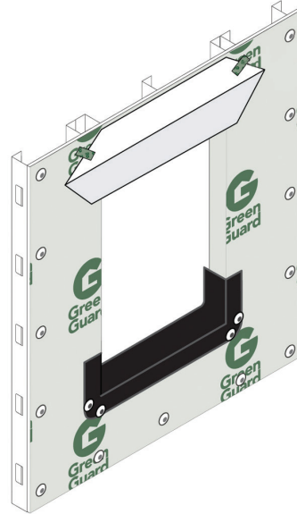
Figure 7 Attachment of Flashing at Corners
