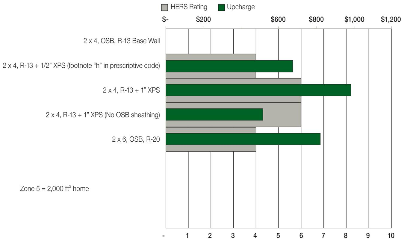
Continuous insulation (Ci) results in increased energy efficiency is illustrated by the increased HERS rating. Ci limits thermal bridging and moves the dew point toward the exterior of the wall cavity reducing energy loss and potential for condensation within the wall cavity.
