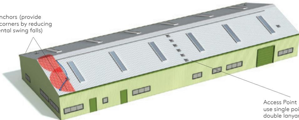
Access Point (first worker should use single point anchors with double lanyard technique only)
