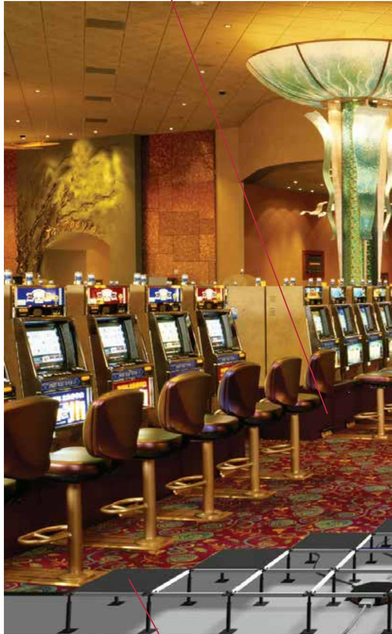
Tate ConCore access floor system - made from over 48% recycled content the welded steel floor panel is filled internally with light-weight cement for the ultimate in strength and acoustic performance.
