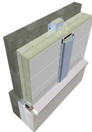
Fig. 7. PAROC Reface panels mounted on to a top hat profile.
